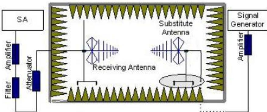
In the chamber, a substitution antenna for the frequency band of interest is placed at the reference point of the chamber. An RF Signal source for the frequency band of interest is connected to the substitution antenna with a cable that has been constructed to not interfere
