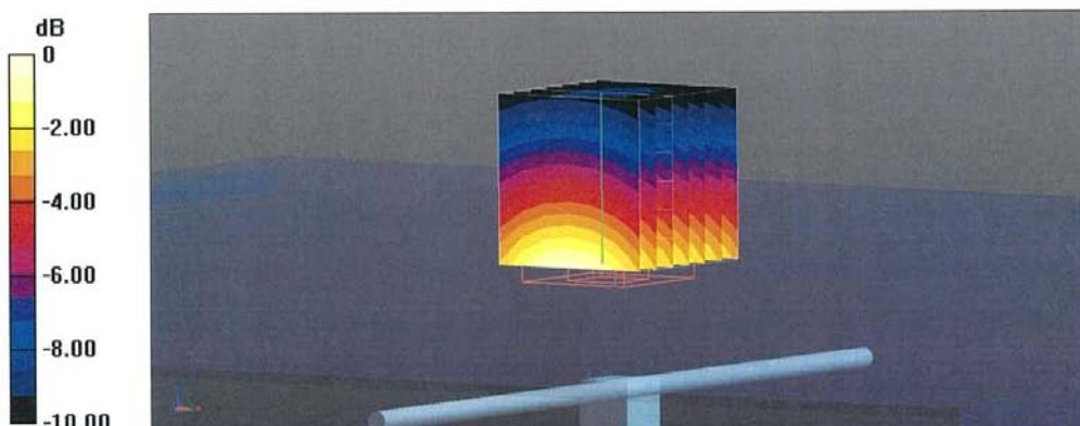
Impedance Measurement Plot for Body TSL
