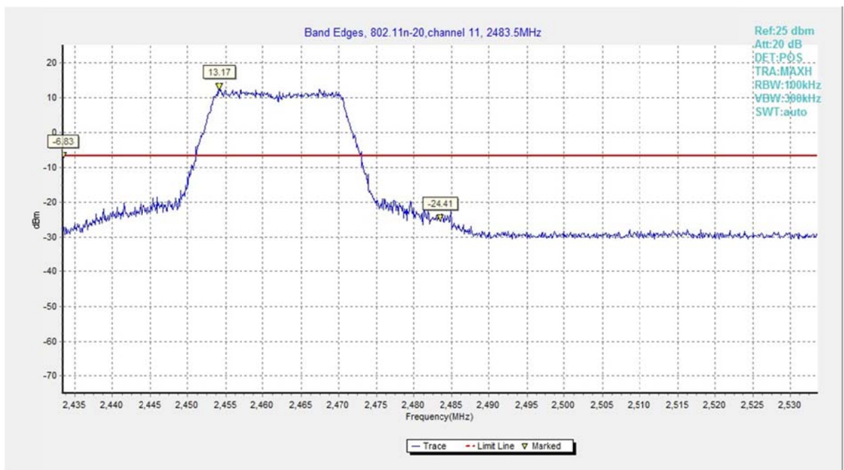
Fig.A.5.6 Band Edges (802.11n-HT20, Ch 11)
