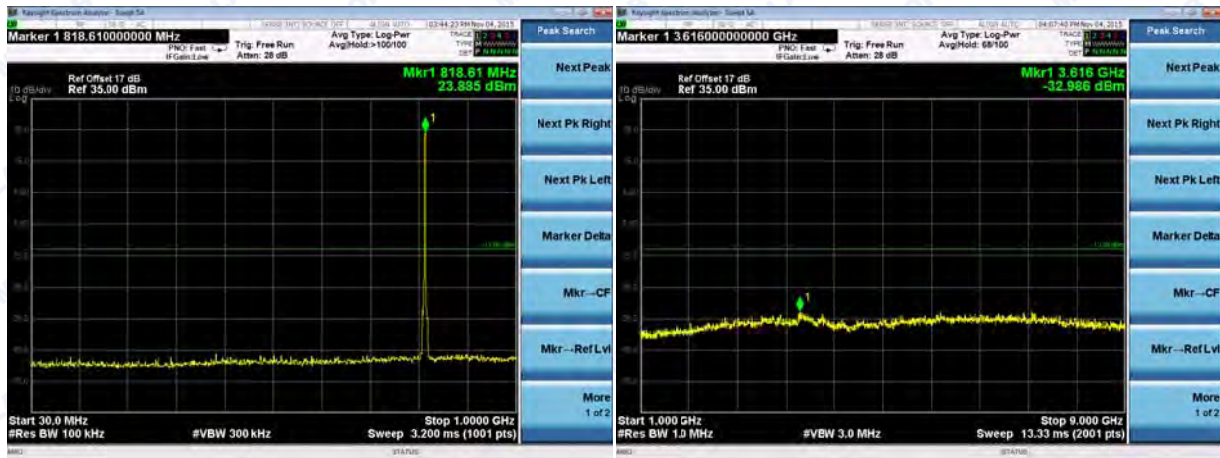
(Plot B20: CDMA BC0 Channel = 500, 30MHz to 9GHz)
