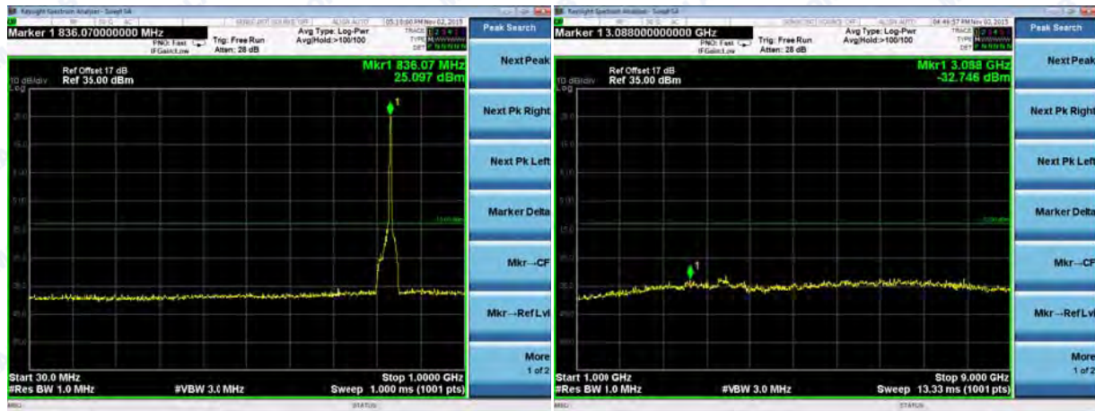
(Plot B5: EVDO 0 BC0 Channel = 384, 30MHz to 9GHz)
