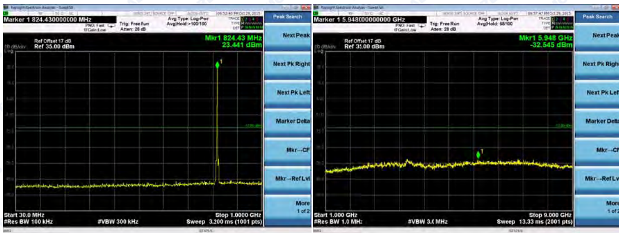
B7: EVDO A BC0 Channel = 1013, 30MHz to 9GHz)
