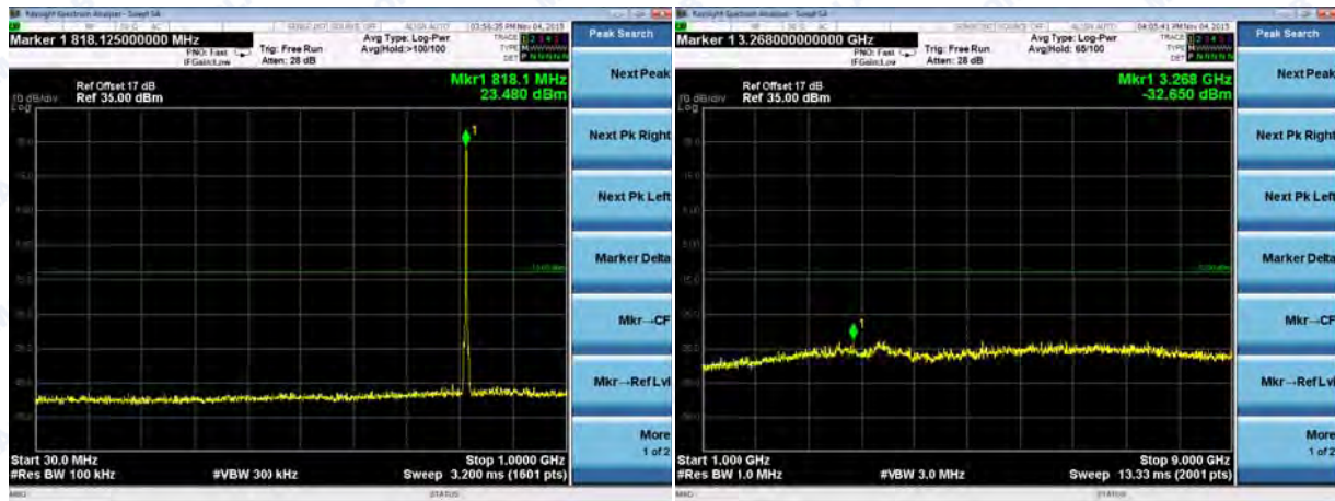
(Plot B23: EVDO 0 BC10 Channel = 500, 30MHz to 9GHz)
