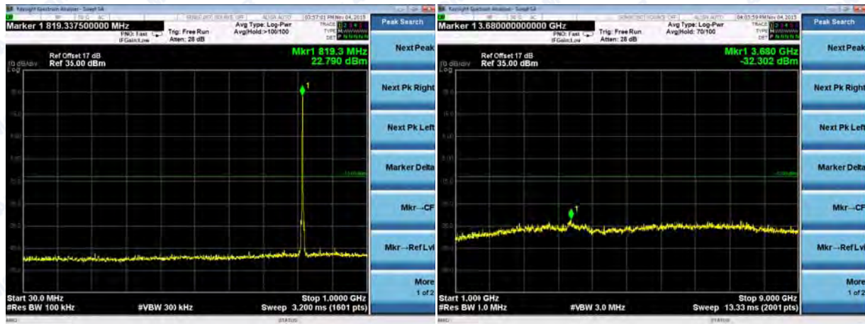
(Plot B24: EVDO 0 BC10 Channel = 550, 30MHz to 9GHz)
