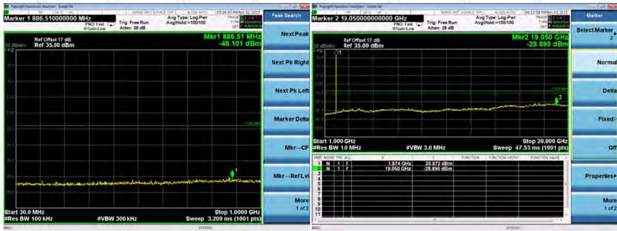
(Plot B14: EVDO 0 BC1 Channel = 600, 30MHz to 20GHz)
