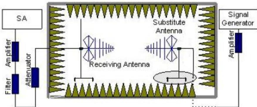
In the chamber, an substitution antenna for the frequency band of interest is placed at the reference point of the chamber. An RF Signal source for the frequency band of interest is connected to the substitution antenna with a cable that has been constructed to not interfere with the radiation pattern of the antenna. A power ( $P_{Mea}$ ) is applied to the input of the substitution antenna, and adjust the level of the signal generator output until the value of the
