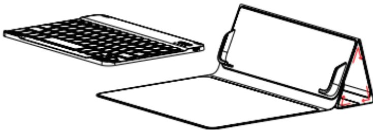
2. Put Tablet into frame and fix.
