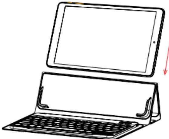
3. Unfold the typefilp to near the Tablet, and then close the typefilp like a book to protect your device.
