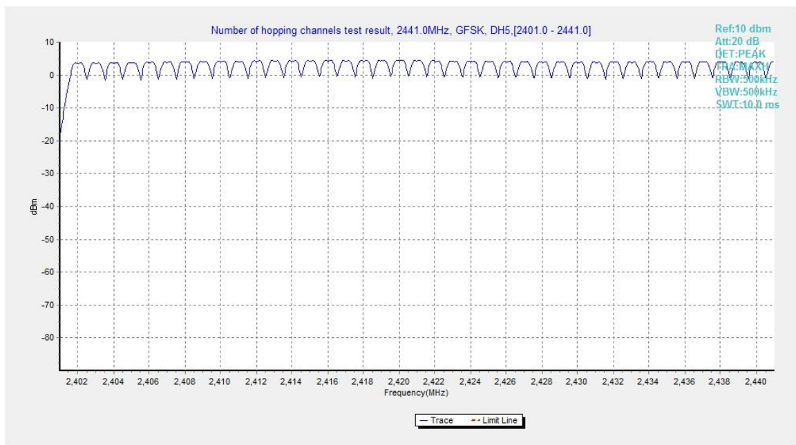
Fig.94. Number of hopping frequencies: GFSK, Channel 0 - 39
