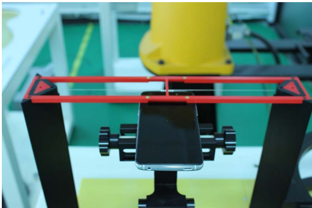
Picture 2: EUT Positioning for RF/T-coil
