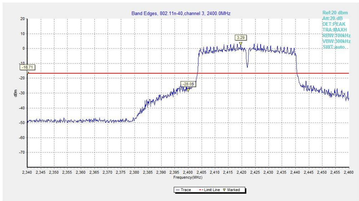
Fig.A.5.7 Band Edges (802.11n-HT40, Ch 3)
