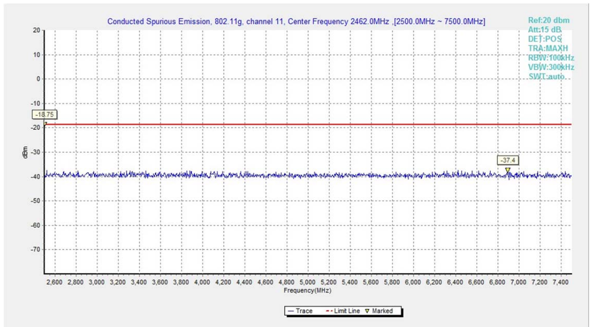
Fig.A.6.1.44 Transmitter Spurious Emission - Conducted (802.11g, Ch11, 2.5 GHz-7.5 GHz)
