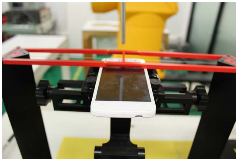
Picture 3: EUT Positioning for T-coil
