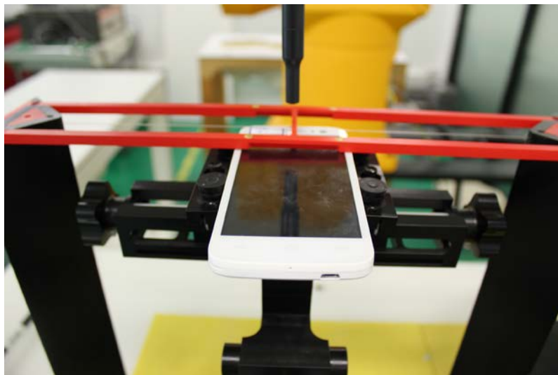
Picture 2: EUT Positioning for RF
