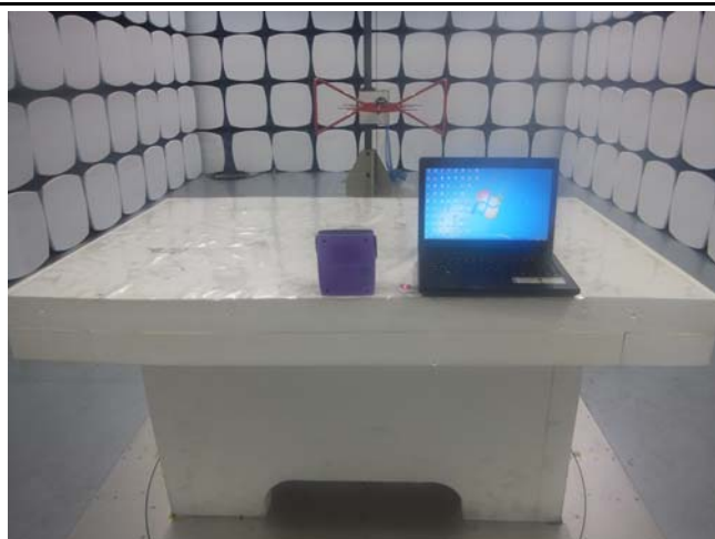
Radiated Spurious Emissions Test Setup Below 1GHz
