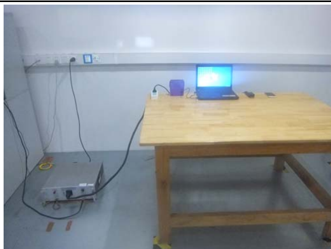
Conducted Emissions Test Setup Front View
