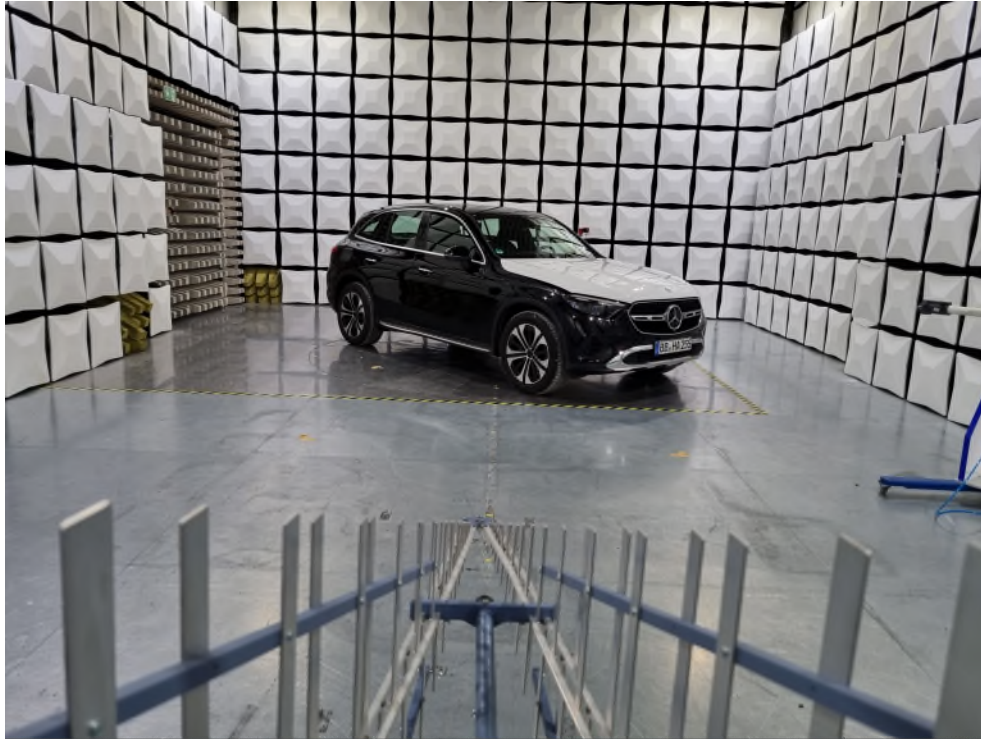
Fig. 5: Set up with EUT for test without absorbers at a car (SUV (X254))
