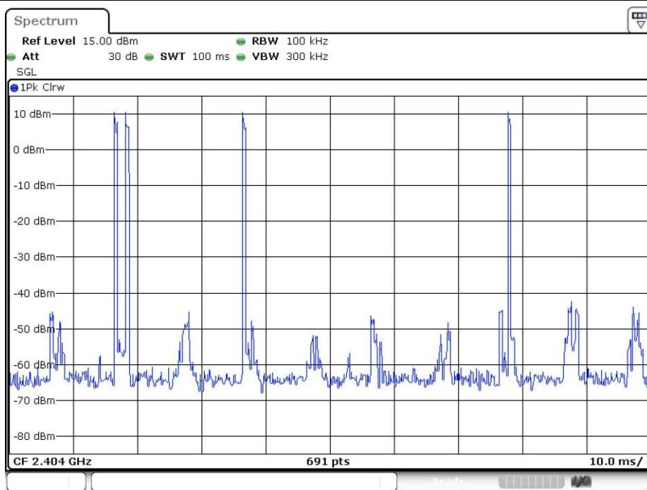
$$20\log (\text{Duty cycle}) = 20\log \frac{4*0.47754 \text{ ms}}{100 \text{ ms}} = -34.38 \text{ dB}$$
