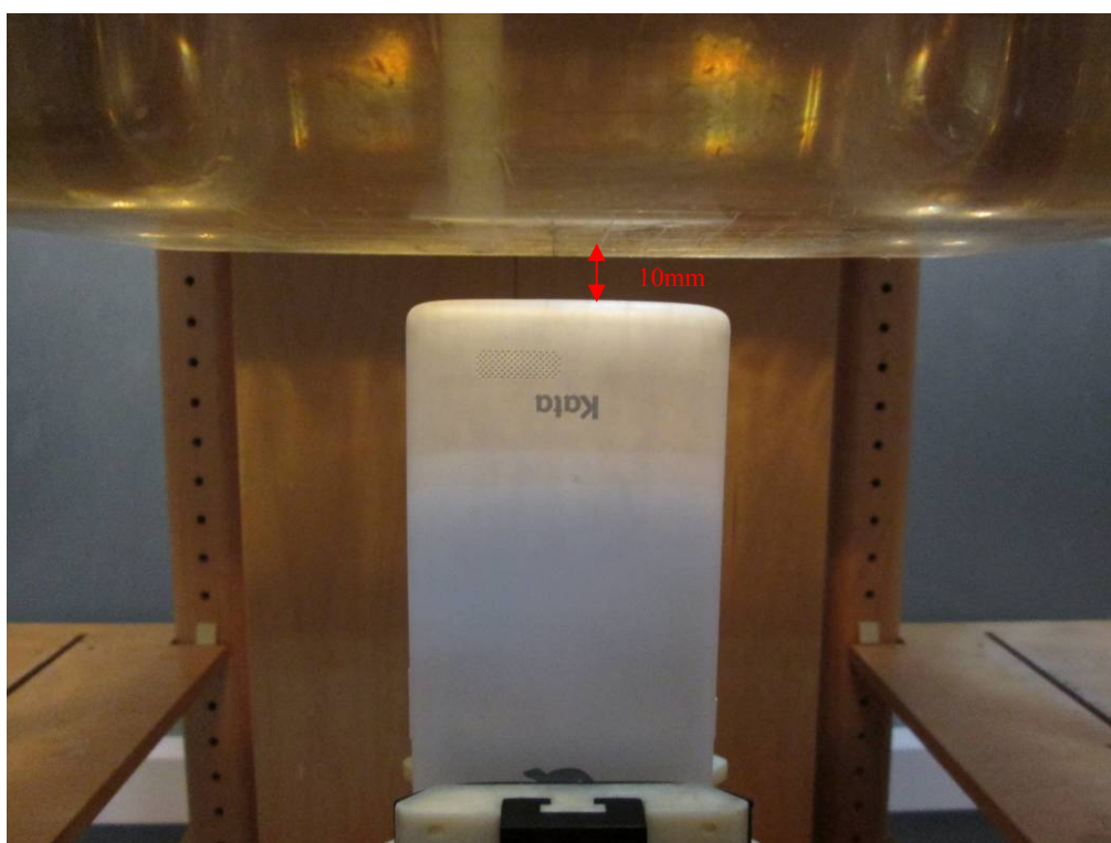
Body-worn Bottom Setup Photo (10mm)
