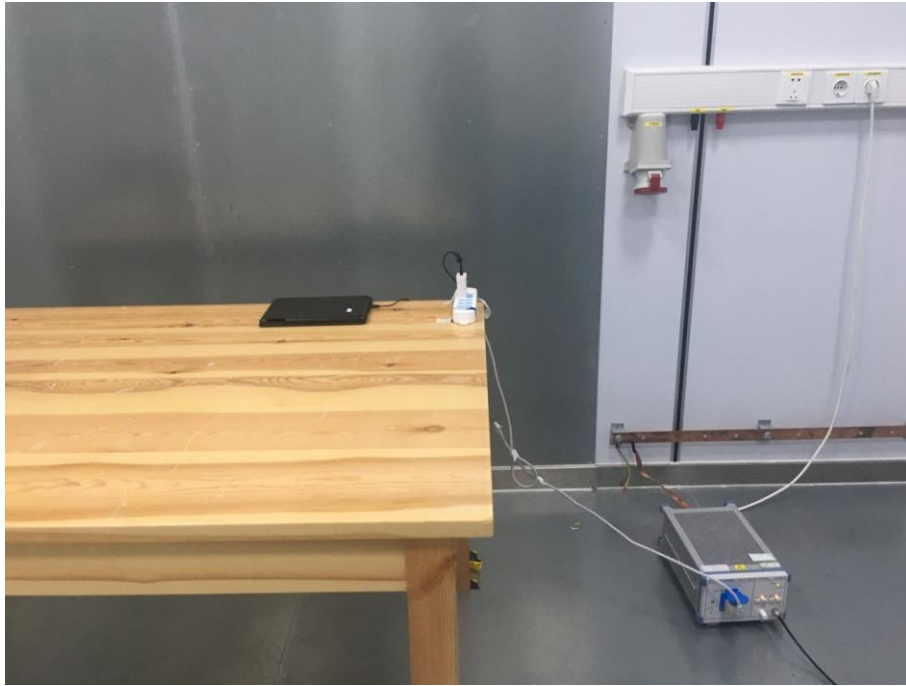
Fig. 5 AC Power Line Conducted emission setup photo
