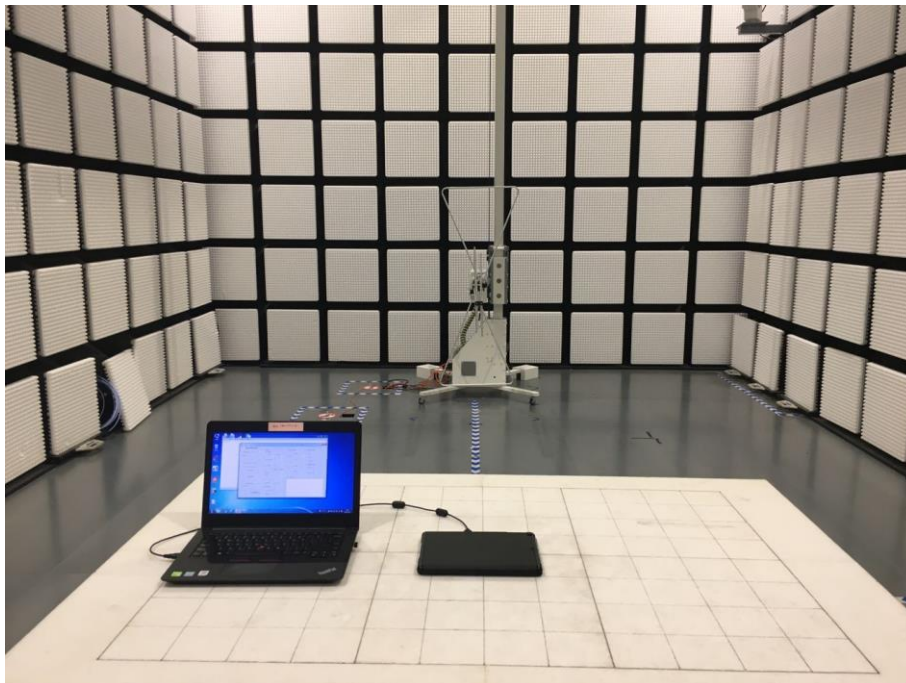
Fig. 2 Radiated emission setup photo(30MHz-1GHz)
