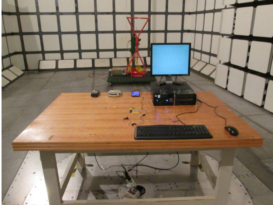
Radiated Emissions – Front View (Below 1 GHz)
