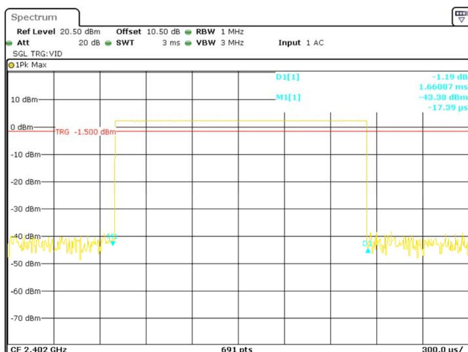
**Pulse time, Middle Channel, DH3**
