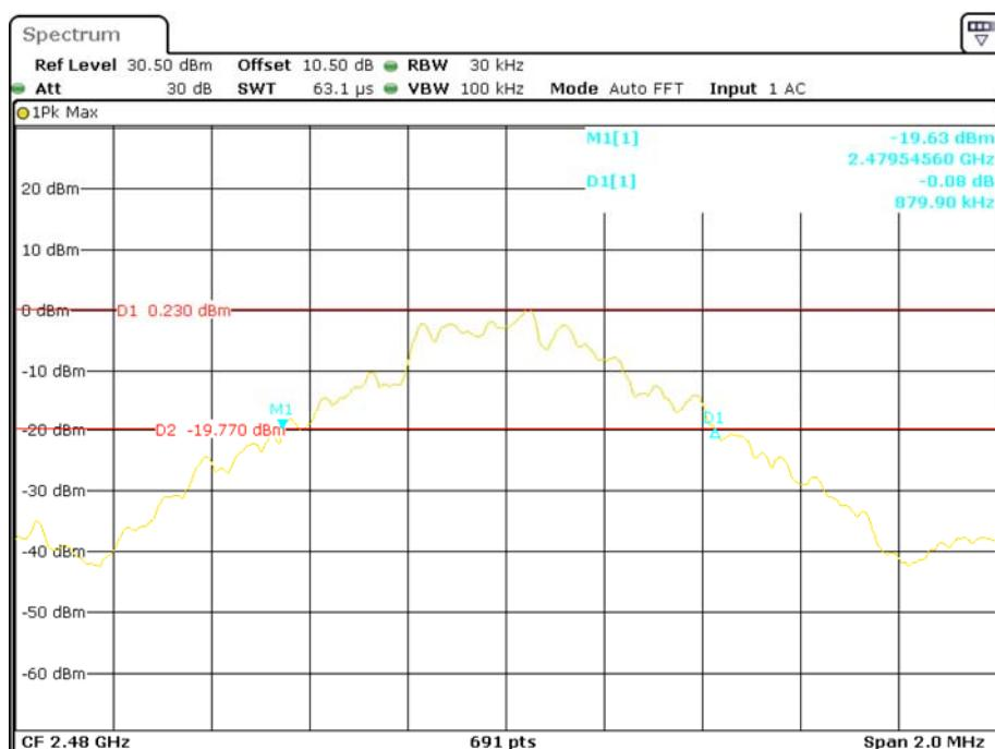
**EDR ( $\pi/4$ -DQPSK): Low Channel**
