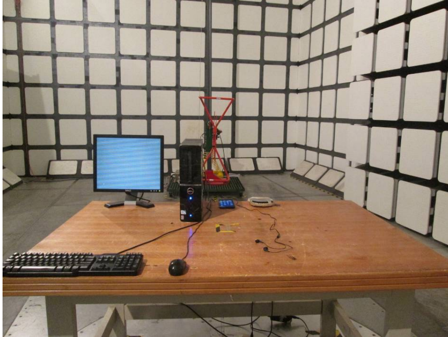
Radiated Emissions – Front View (Below 1 GHz)
