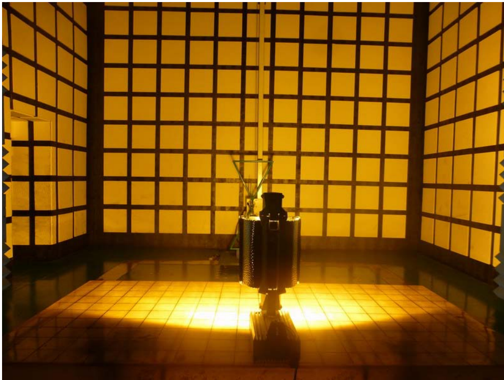
Photograph 4: Radiated Emission Test Configuration, (30-1000MHz), Back
