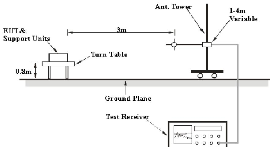
The radiated emission tests was performed in the 3 meters chamber test site, using the setup accordance with the ANSI C63.4-2003. The specification used was the FCC Part 15.109, Class B limits.
