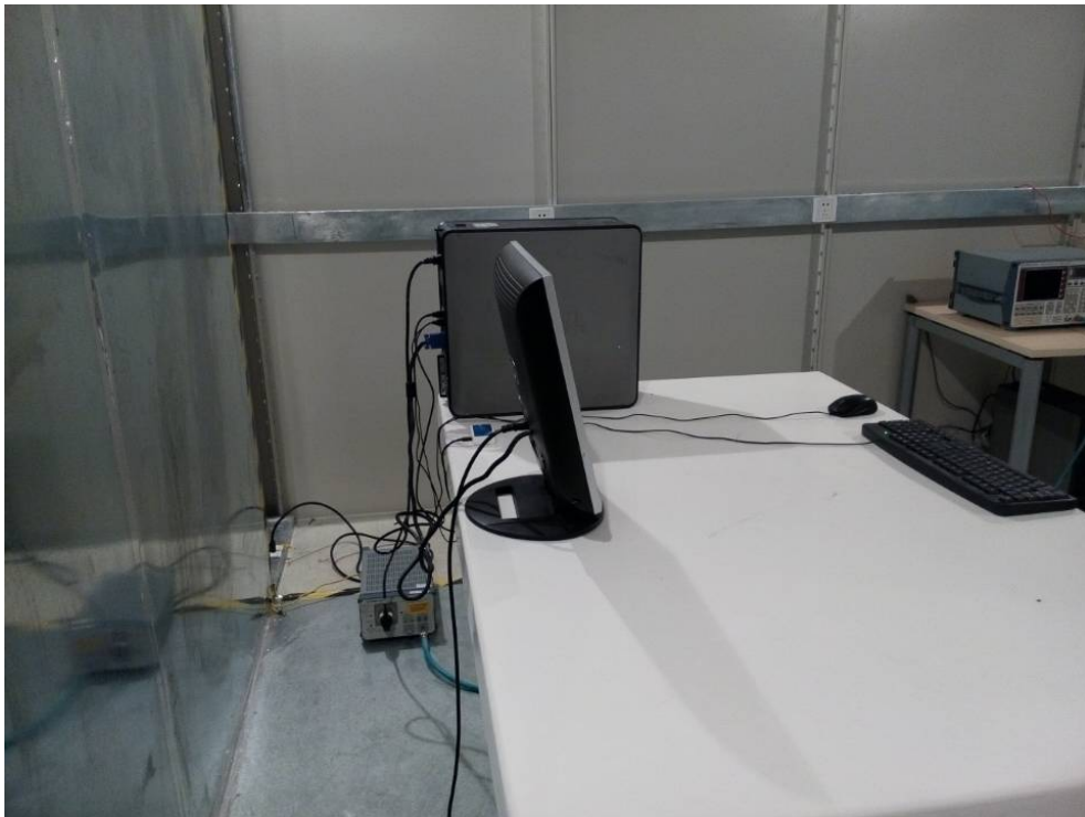
Conducted Emissions - Side View
