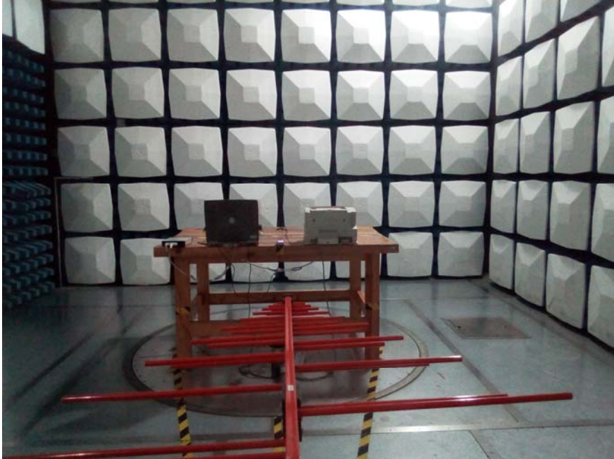
Radiated Emission Below 1GHz – Rear View
