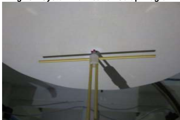
Fig.10.2 Photo of Dipole setup
