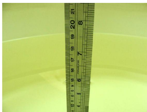
Fig 7.2 Photo of Liquid Height for Body SAR
