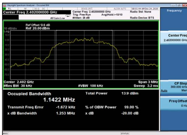
20dB Bandwidth: 8DPSK,2480MHz,3DH5
