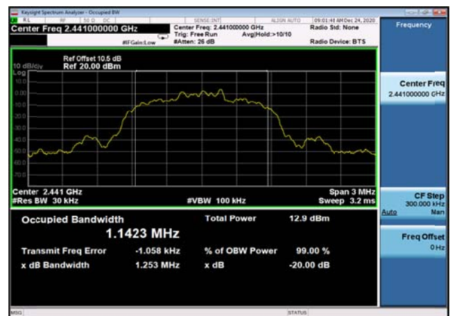
20dB Bandwidth: 8DPSK,2441MHz,3DH5
