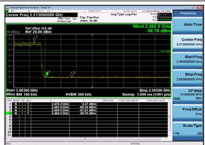
Conducted Emission: 8DPSK,2480,3DH5 ,Band Edge
