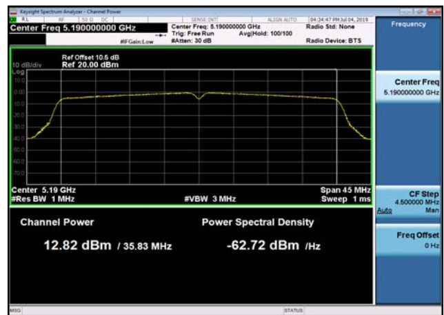
U-NII-1 Output Power-802.11a(20MHz) ,5180MHz
