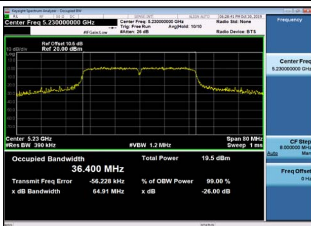
U-NII-1 26dB Bandwidth-802.11n(40MHz) ,5230MHz,Ant1
