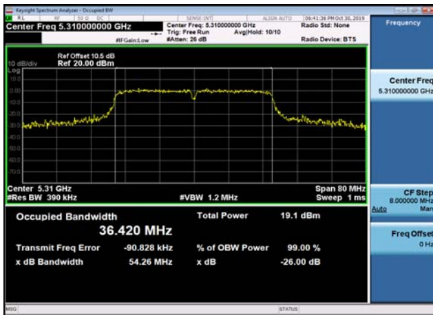
U-NII-2a 26dB Bandwidth-802.11a(20MHz),5300MHz,Ant1
