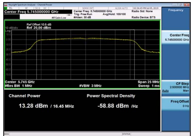
U-NII-3 Output Power-802.11a(20MHz) ,5825MHz
