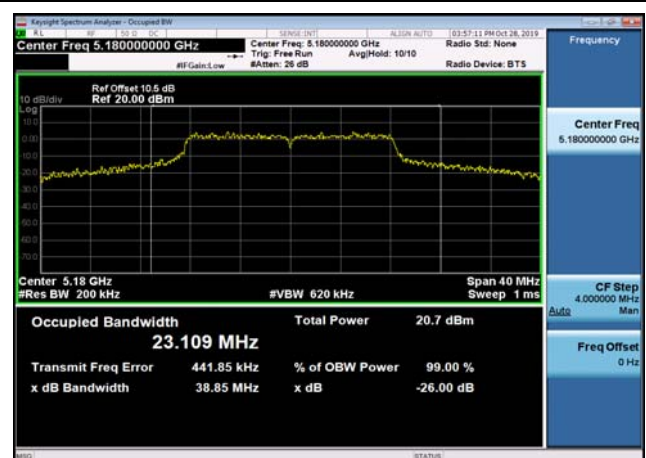
U-NII-1 26dB Bandwidth-802.11a(20MHz) ,5180MHz,Ant1
