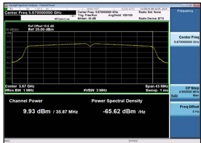
U-NII-2c Output Power-802.11a(20MHz) ,5600MHz
