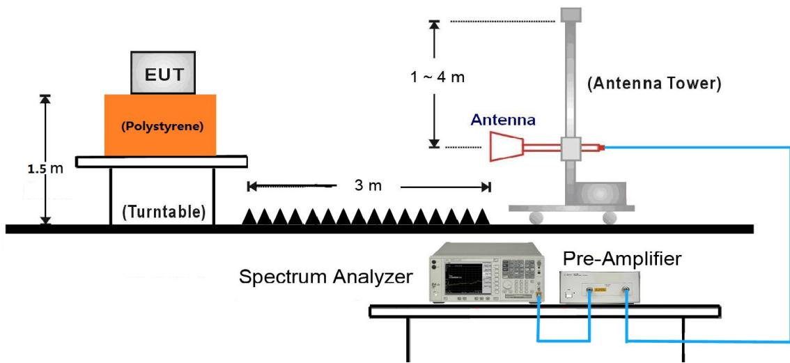
18GHz ~25GHz Test Setup:
