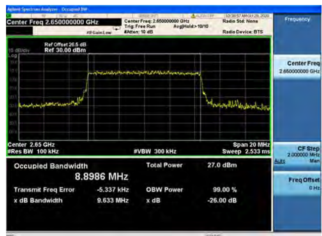
Band41 / 10MHz / High CH / 16QAM
