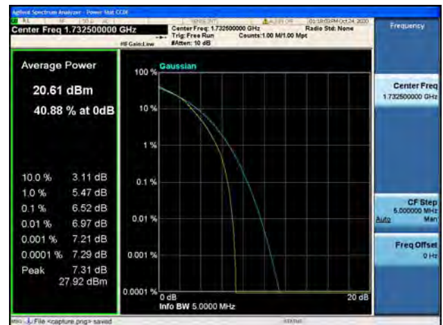
Band4 / 5MHz / High CH / 16QAM
