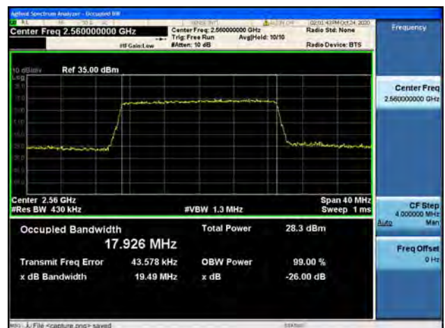
Band7 / 20MHz / High CH / 16QAM
