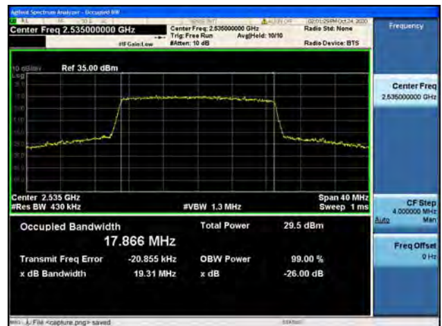
Band7 / 20MHz / High CH / 16QAM
