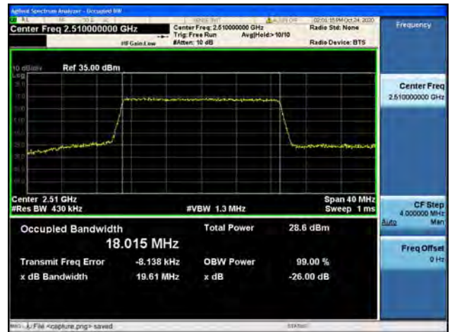
Band7 / 20MHz / Mid CH / 16QAM
