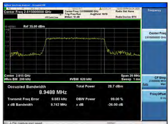
Band38 / 10MHz / High CH / 16QAM
