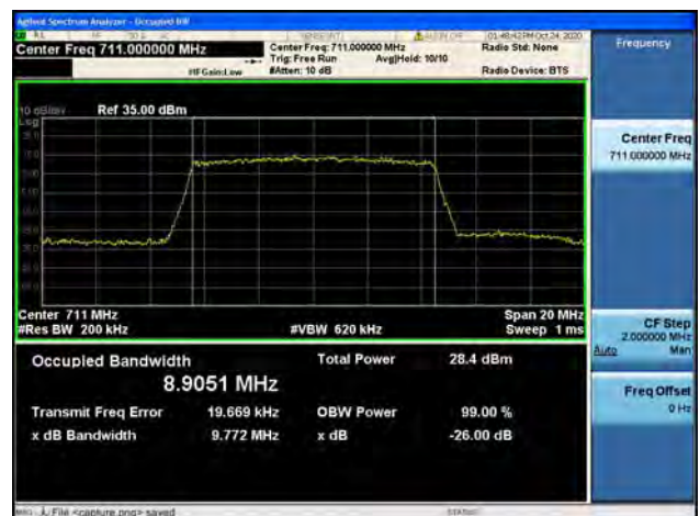
Band12 / 10MHz / High CH / 16QAM
