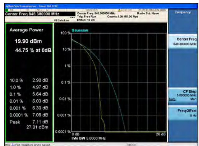
Band5 / 1.4MHz / High CH / 16QAM
