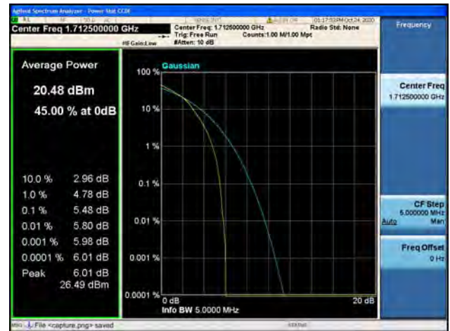
Band4 / 5MHz / Mid CH / 16QAM
