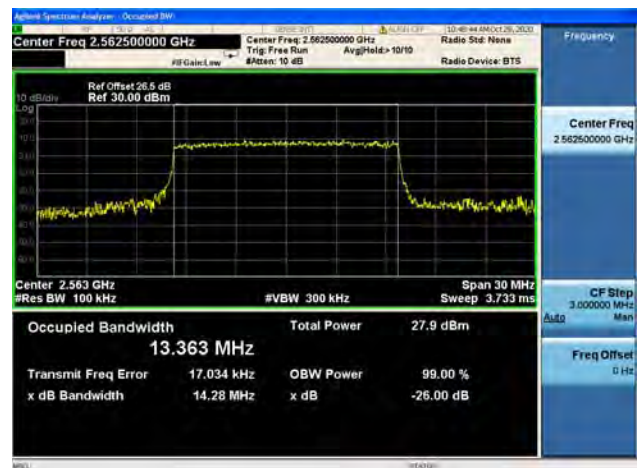
Band41 / 15MHz / High CH / 16QAM
