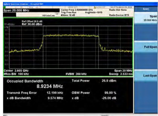
Band41 / 10MHz / High CH / 16QAM
