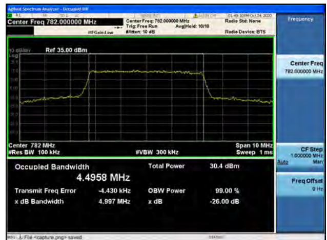
Band13 / 5MHz / High CH / 16QAM
