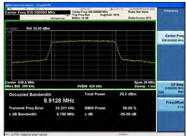
Band5 / 10MHz / High CH / 16QAM
