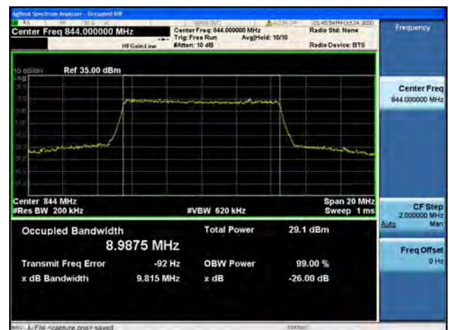
Band5 / 10MHz / High CH / 16QAM
