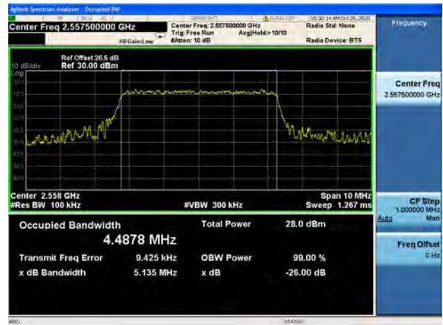
Band41 / 5MHz / Mid CH / 16QAM
