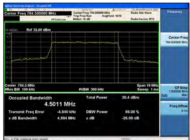
Band13 / 5MHz / High CH / 16QAM
