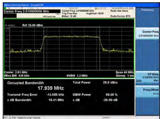
Band38 / 20MHz / High CH / 16QAM
