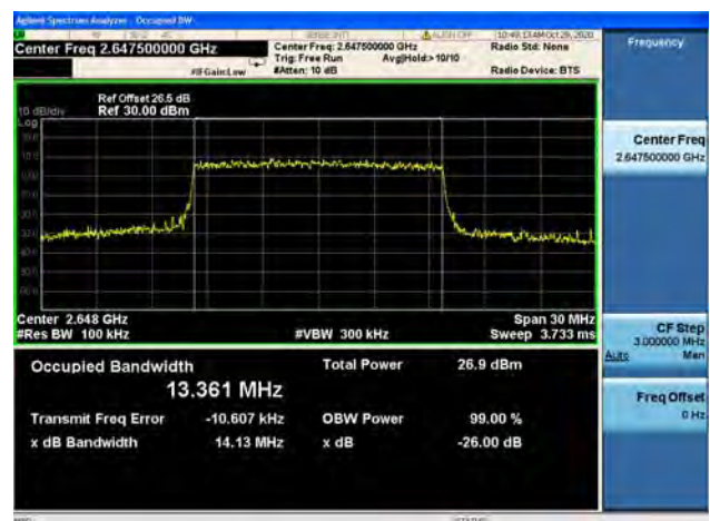
Band41 / 15MHz / High CH / 16QAM
