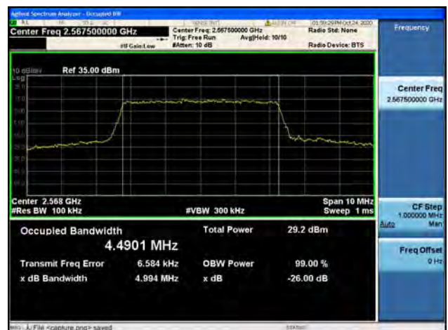
Band7 / 5MHz / High CH / 16QAM
