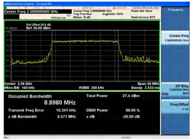
Band41 / 10MHz / Mid CH / 16QAM
