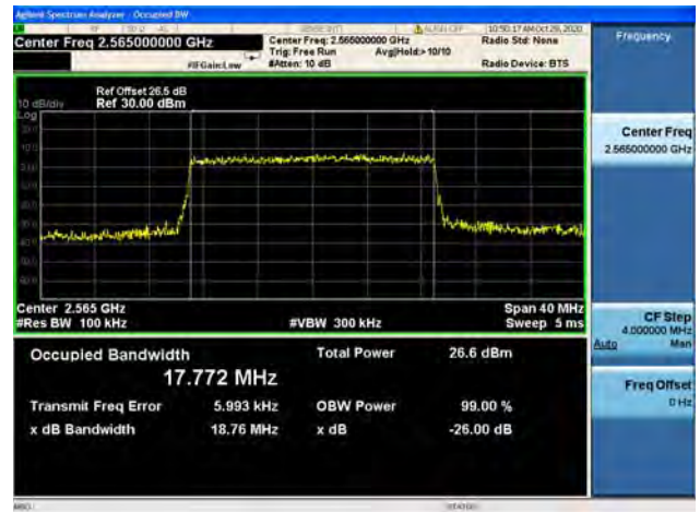
Band41 / 20MHz / Mid CH / 16QAM
