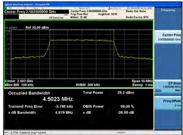
Band7 / 5MHz / Mid CH / 16QAM
