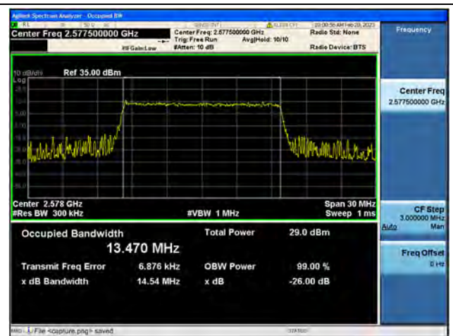
Band38 / 15MHz / 16QAM/ Low CH
