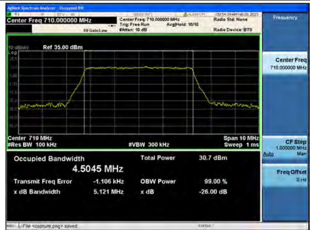
Band17 / 5MHz / QPSK/ Mid CH
