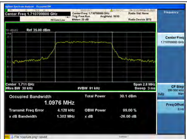
Band4 / 1.4MHz / 16QAM/ Low CH
