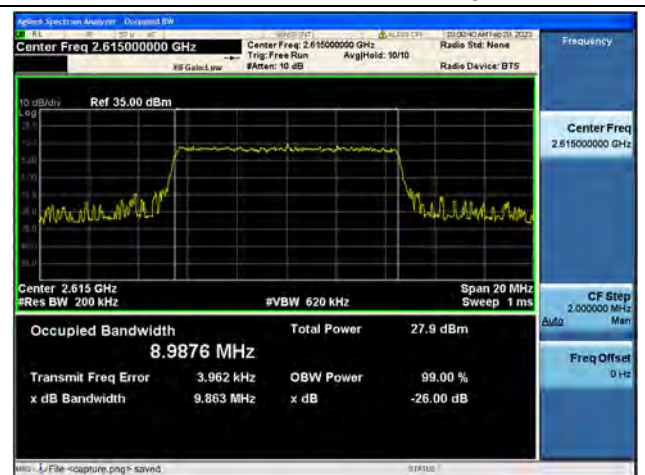
Band38 / 10MHz / 64QAM/ High CH
