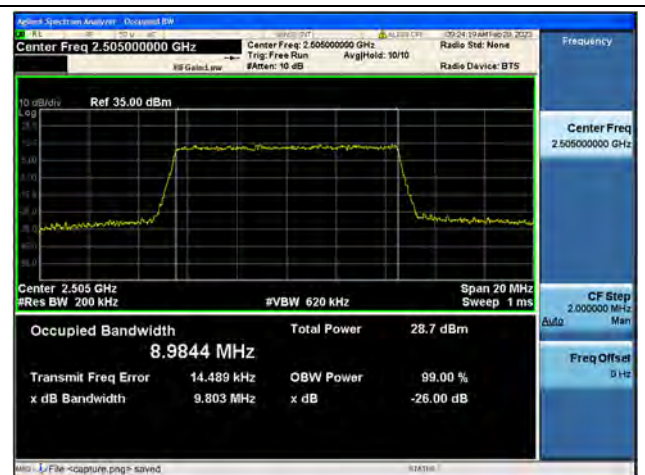
Band7 / 10MHz / 64QAM / Low CH
