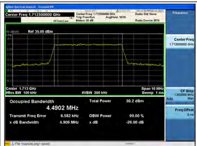
Band4 / 5MHz / 16QAM/ Low CH
