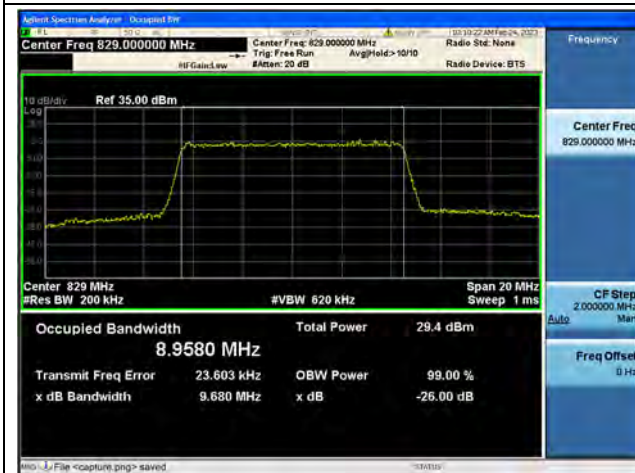
Band5 / 10MHz / 16QAM/ Low CH
