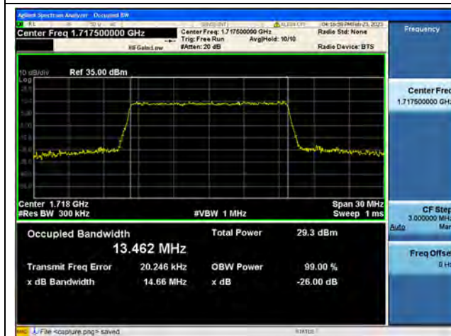
Band4 / 15MHz / 64QAM/ Low CH
