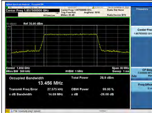
Band2 / 15MHz / 64QAM/ Low CH
