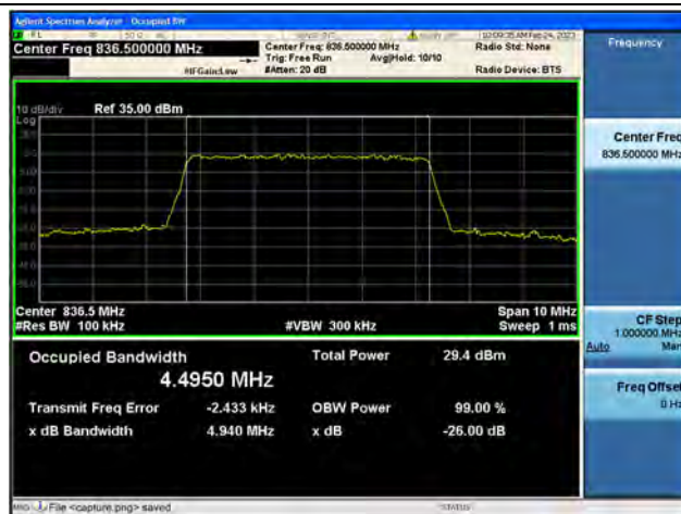
Band5 / 5MHz / 16QAM/ Mid CH
