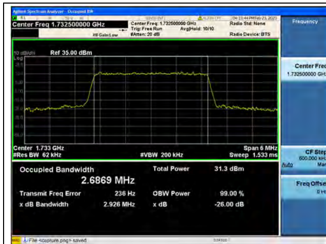
Band4 / 3MHz / QPSK/ Mid CH
