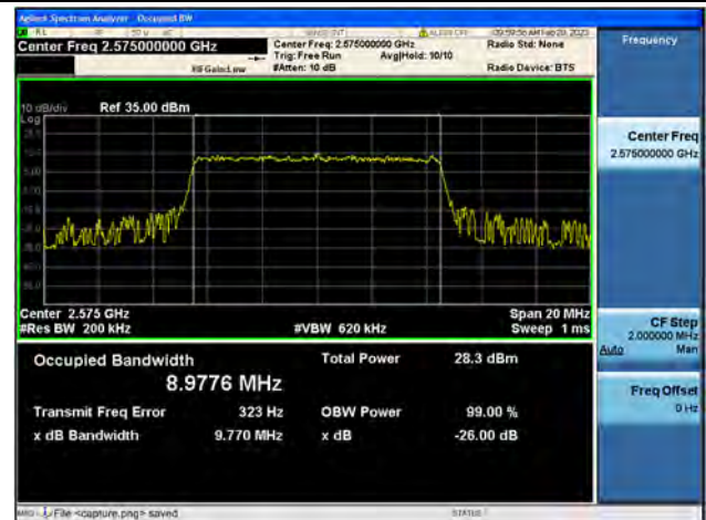
Band38 / 10MHz / 64QAM/ Low CH
