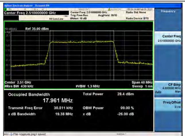
Band7 / 20MHz / 64QAM/ Low CH
