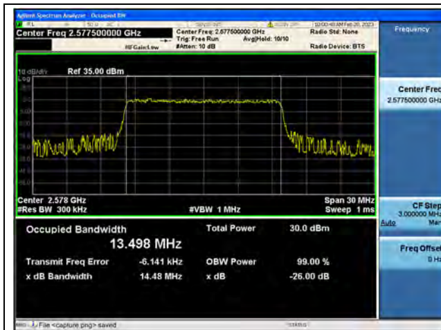
Band38 / 15MHz / QPSK/ Low CH
