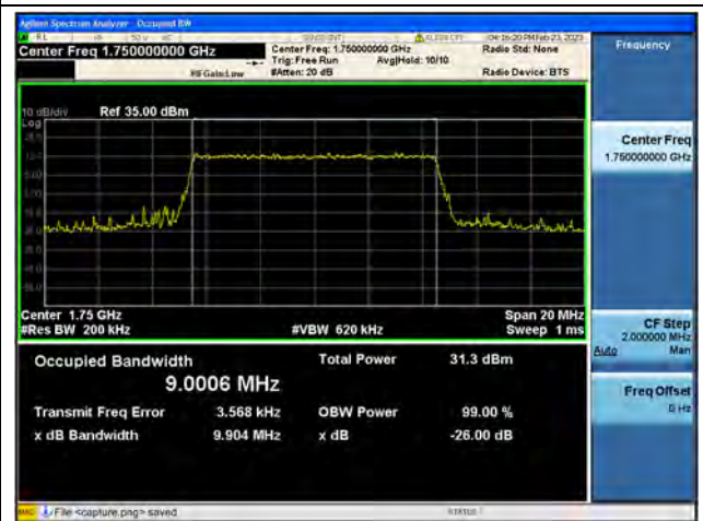
Band4 / 10MHz / QPSK/ High CH
