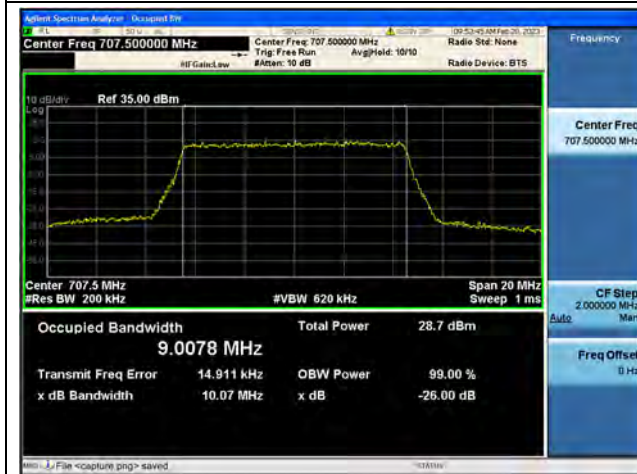
Band12 / 10MHz / 64QAM/ Mid CH
