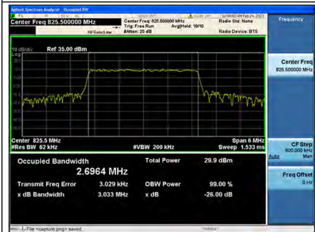
Band5 / 3MHz / 16QAM/ Low CH
