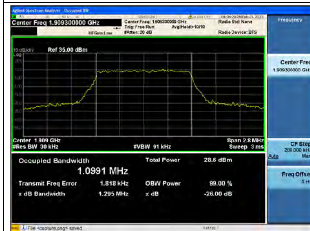
Band2 / 1.4MHz / 64QAM/ High CH
