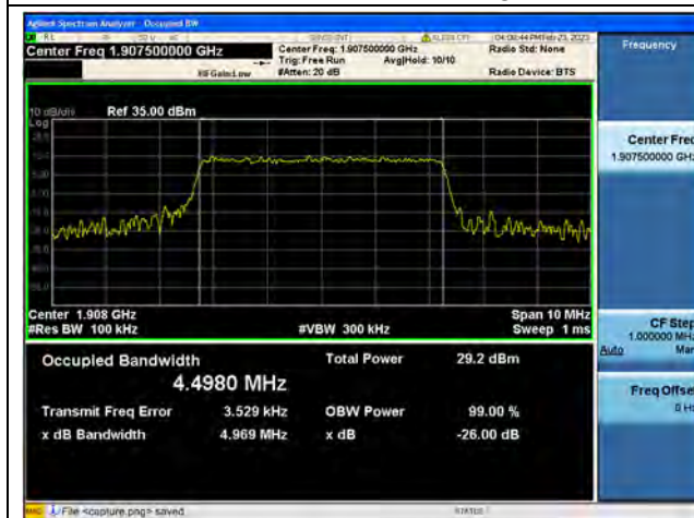
Band2 / 5MHz / 64QAM/ High CH
