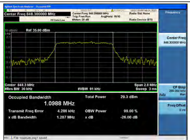
Band5 / 1.4MHz / 16QAM/ High CH
