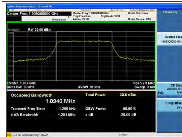
Band2 / 1.4MHz / QPSK/ High CH
