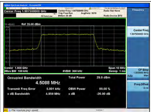
Band2 / 5MHz / 16QAM/ High CH
