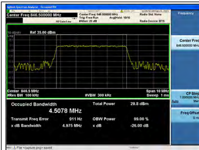
Band5 / 5MHz / QPSK/ High CH
