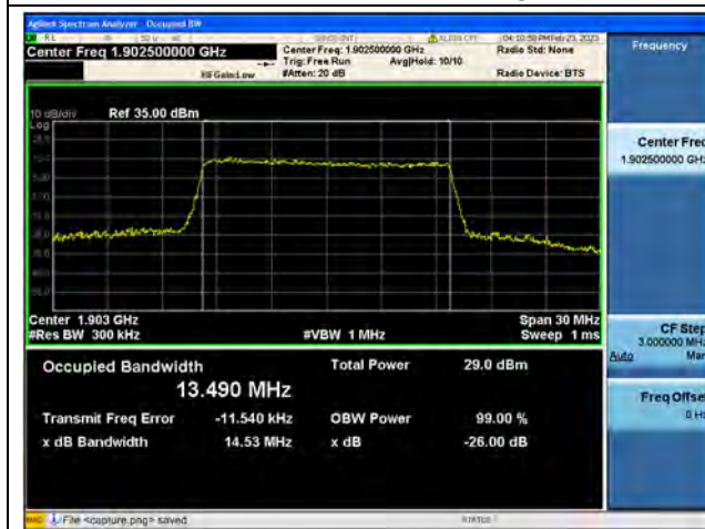
Band2 / 15MHz / 64QAM/ High CH
