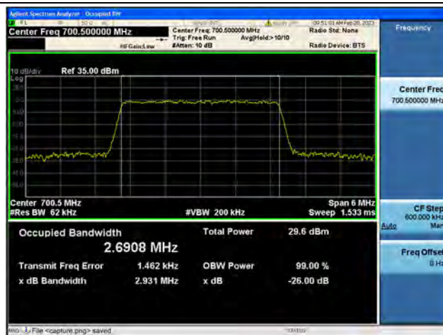
Band12 / 3MHz / 16QAM/ Low CH
