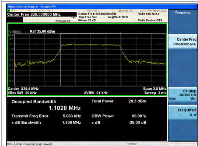
Band5 / 1.4MHz / 16QAM/ Mid CH
