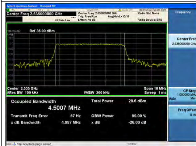
Band7 / 5MHz / 16QAM/ Mid CH
