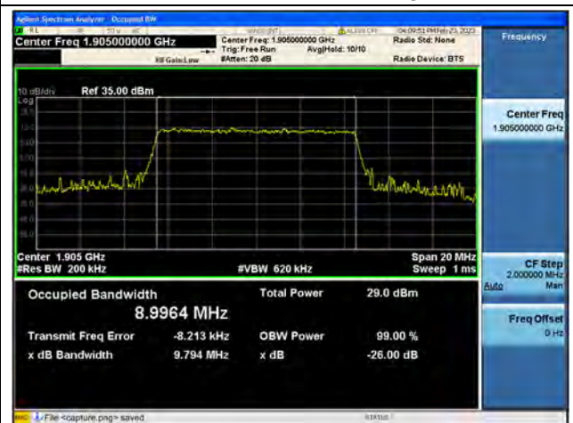
Band2 / 10MHz / 64QAM/ High CH
