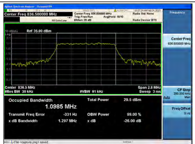
Band5 / 1.4MHz / 64QAM/ Mid CH
