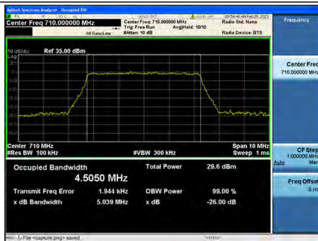
Band17 / 5MHz / 16QAM/ Mid CH
