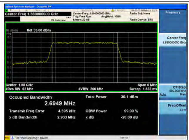
Band2 / 3MHz / 16QAM/ Mid CH
