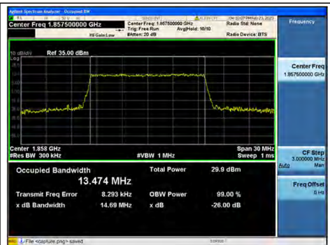
Band2 / 15MHz / 16QAM/ Low CH
