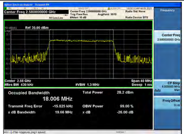
Band38 / 20MHz / 64QAM/ Low CH
