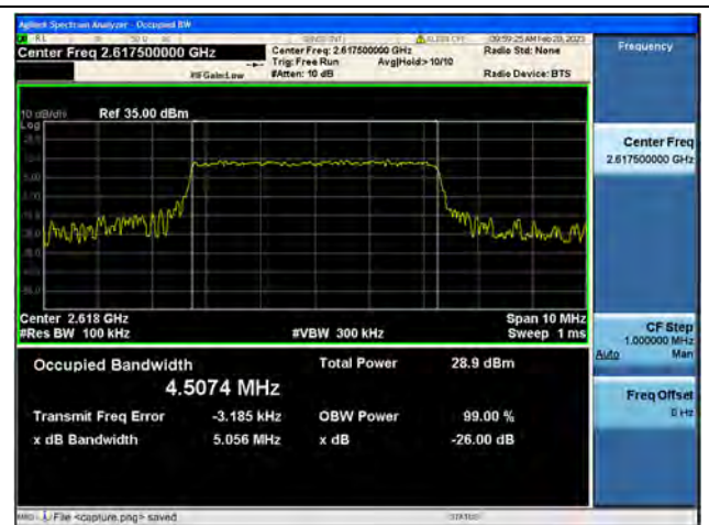
Band38 / 5MHz / 16QAM/ High CH
