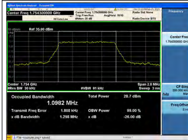
Band4 / 1.4MHz / 64QAM/ High CH
