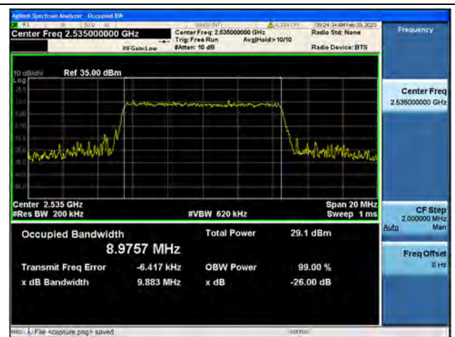
Band7 / 10MHz / 16QAM/ Mid CH
