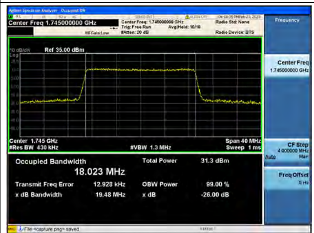
Band4 / 20MHz / QPSK/ High CH
