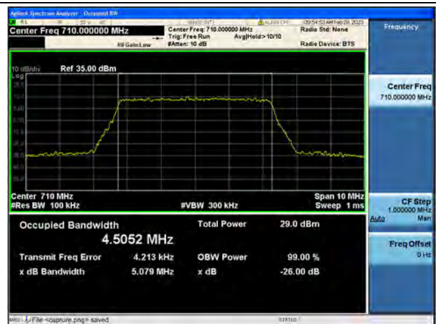
Band17 / 5MHz / 64QAM/ Mid CH
