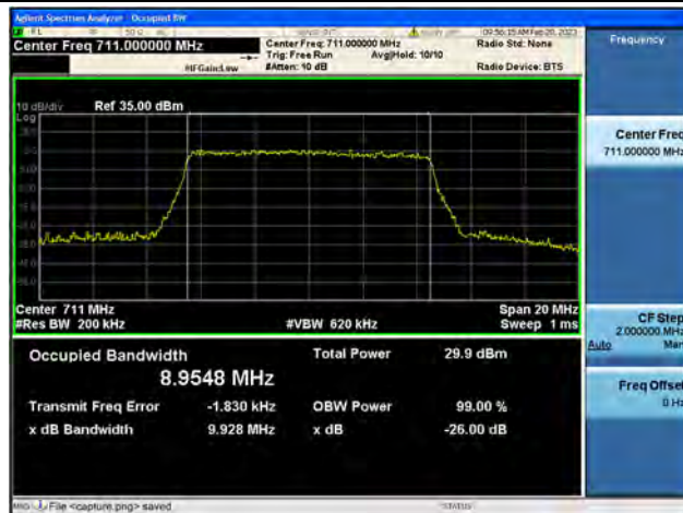
Band17 / 10MHz / 16QAM/ High CH
