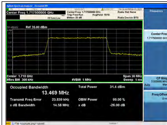
Band4 / 15MHz / QPSK/ Low CH
