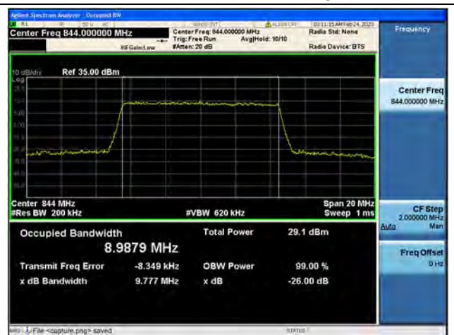
Band5 / 10MHz / 64QAM/ High CH
