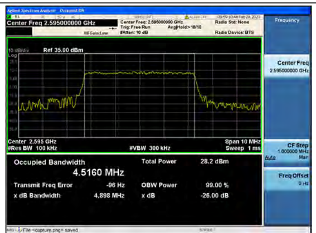
Band38 / 5MHz / 64QAM/ Mid CH
