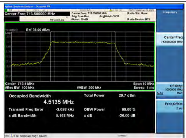
Band12 / 5MHz / 16QAM/ High CH
