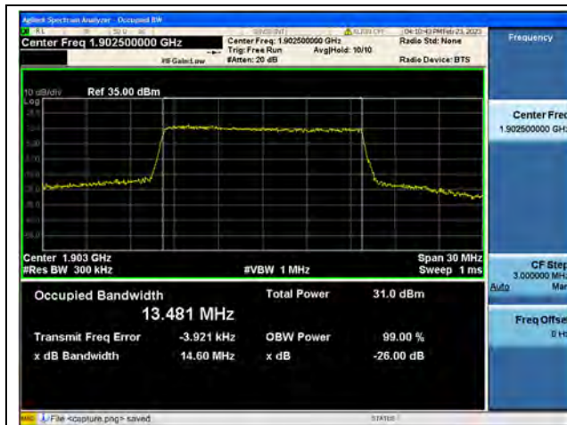
Band2 / 15MHz / QPSK/ High CH
