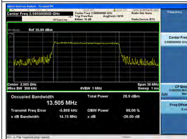
Band38 / 15MHz / 16QAM/ Mid CH
