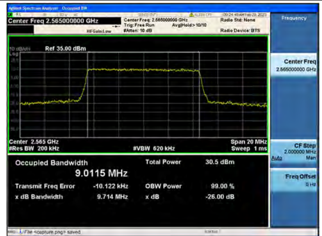
Band7 / 10MHz / QPSK/ High CH
