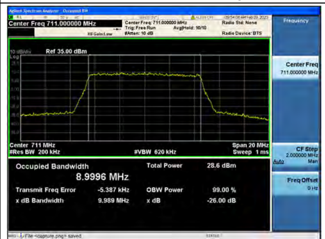
Band12 / 10MHz / 64QAM/ High CH
