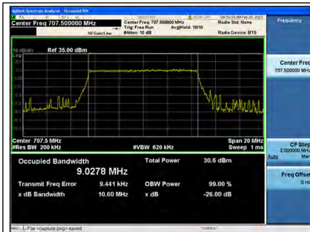
Band12 / 10MHz / QPSK/ Mid CH
