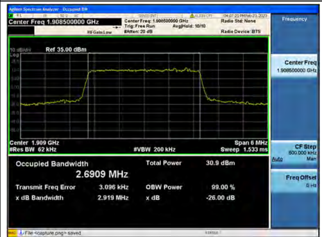
Band2 / 3MHz / QPSK/ High CH
