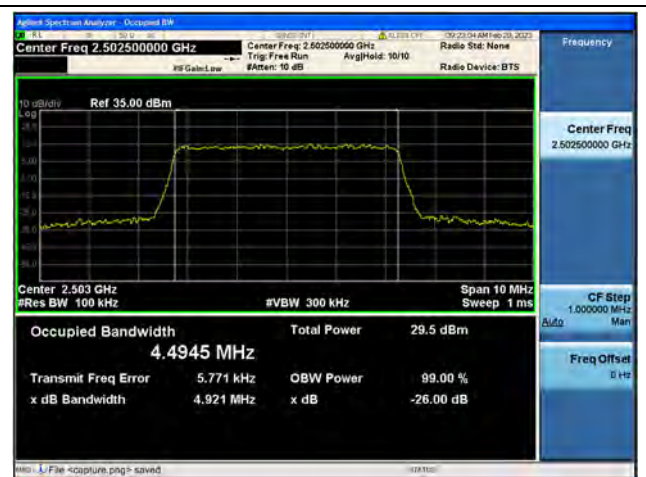
Band7 / 5MHz / 16QAM/ Low CH
