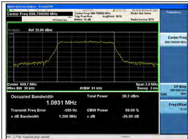
Band12 / 1.4MHz / QPSK/ Low CH
