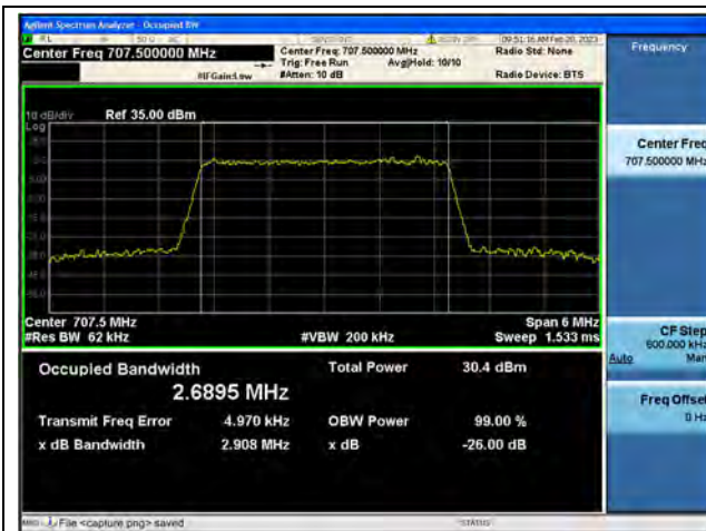
Band12 / 3MHz / QPSK/ Mid CH
