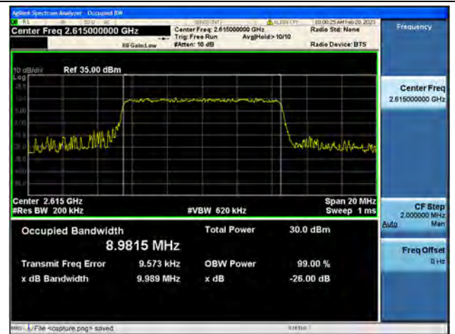
Band38 / 10MHz / QPSK/ High CH
