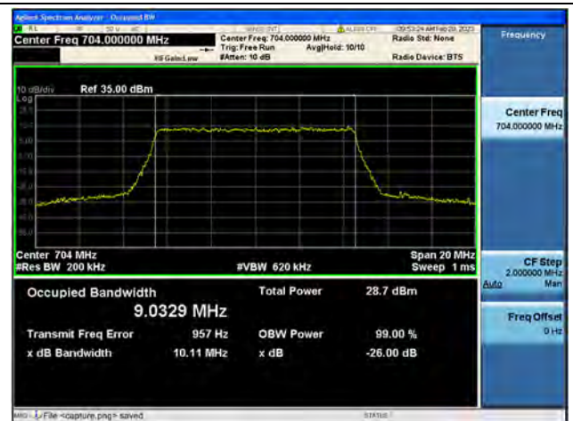
Band12 / 10MHz / 64QAM/ Low CH
