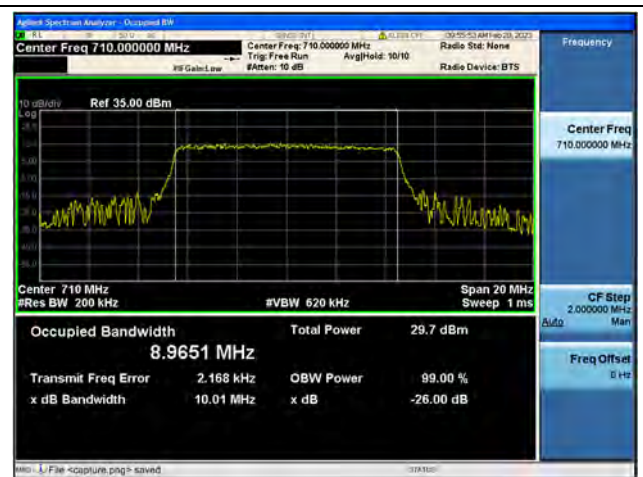
Band17 / 10MHz / 16QAM/ Mid CH
