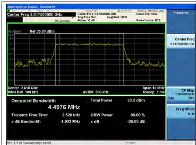
Band38 / 5MHz / QPSK/ High CH
