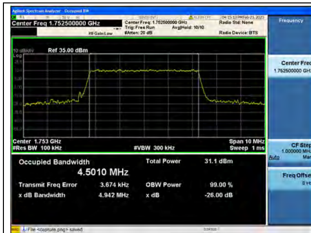
Band4 / 5MHz / QPSK/ High CH
