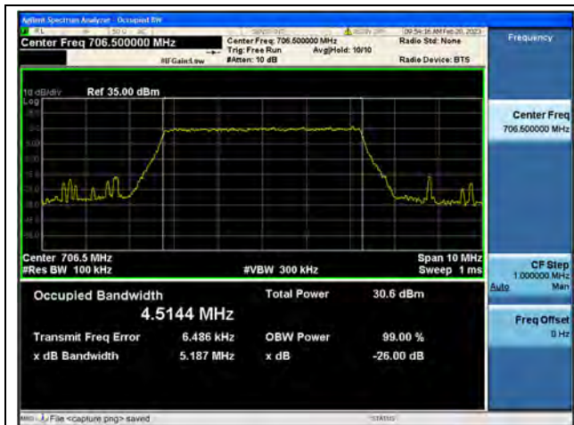
Band17 / 5MHz / QPSK/ Low CH
