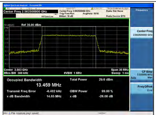
Band7 / 15MHz / 16QAM/ High CH
