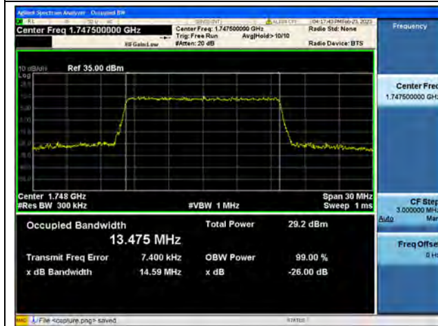
Band4 / 15MHz / 64QAM/ High CH
