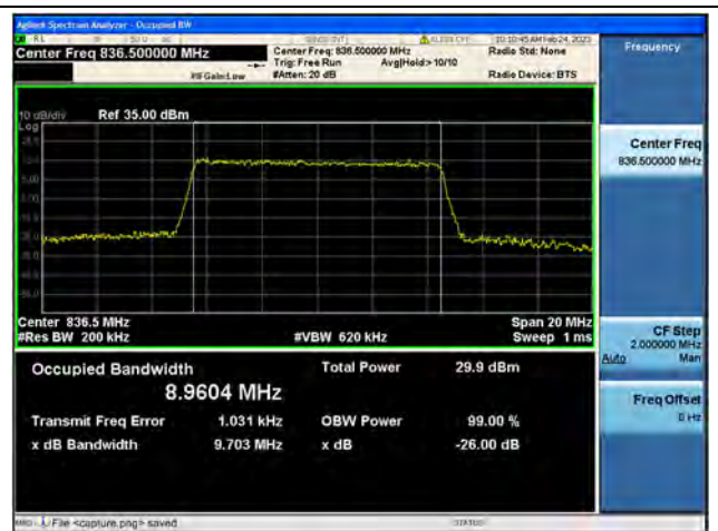
Band5 / 10MHz / 16QAM/ Mid CH
