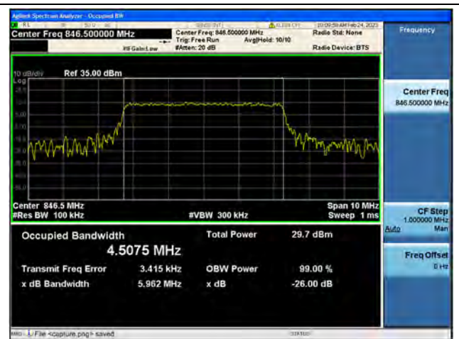
Band5 / 5MHz / 16QAM/ High CH
