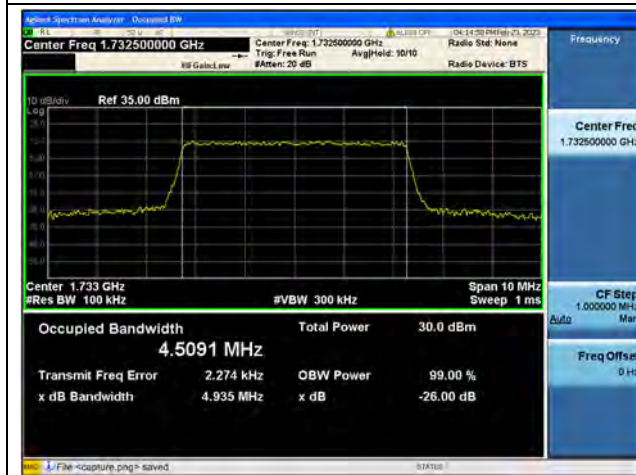
Band4 / 5MHz / 16QAM/ Mid CH
