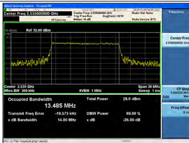
Band7 / 15MHz / 16QAM/ Mid CH
