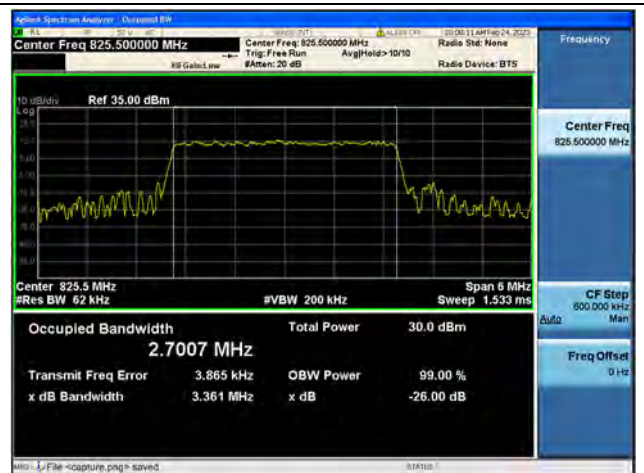
Band5 / 3MHz / 64QAM/ Low CH
