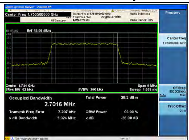
Band4 / 3MHz / 64QAM/ High CH
