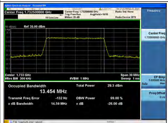
Band4 / 15MHz / 64QAM/ Mid CH
