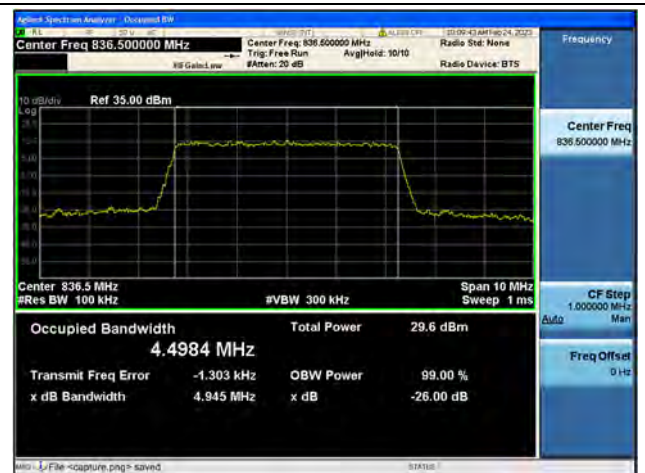
Band5 / 5MHz / 64QAM/ Mid CH
