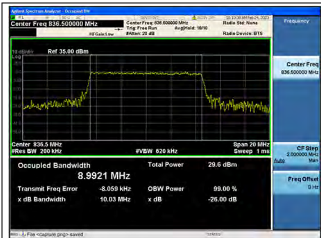
Band5 / 10MHz / QPSK/ Mid CH
