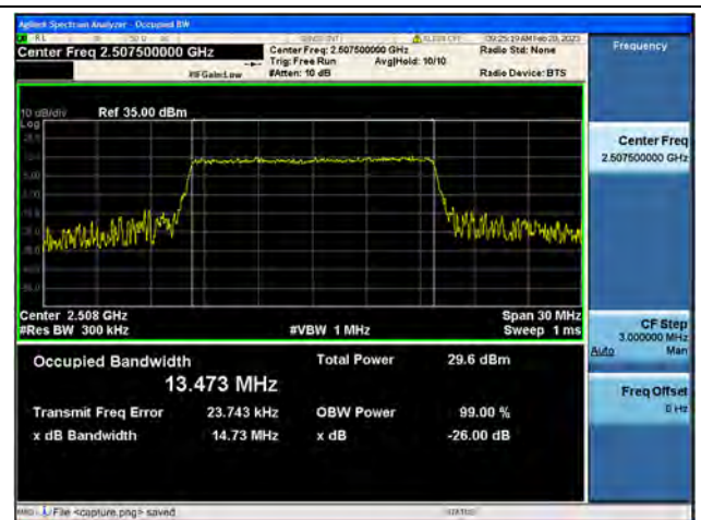
Band7 / 15MHz / 16QAM/ Low CH
