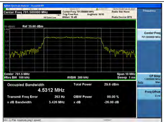
Band12 / 5MHz / 16QAM/ Low CH
