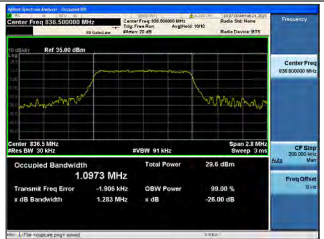
Band5 / 1.4MHz / QPSK/ Mid CH
