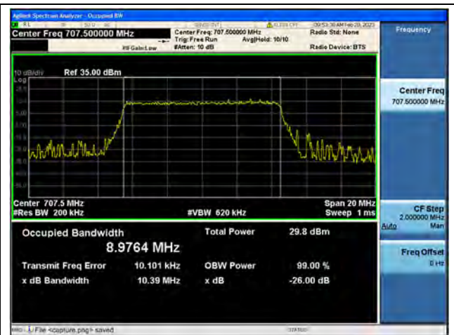
Band12 / 10MHz / 16QAM/ Mid CH
