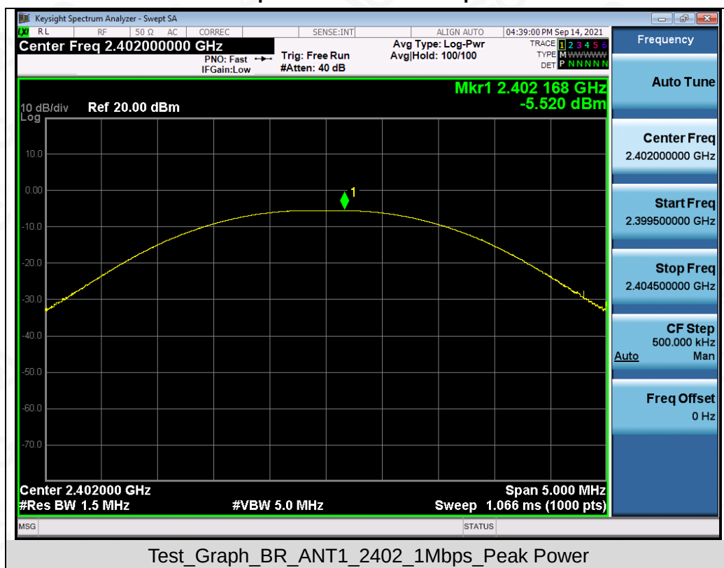
Test Graphs of Conducted Output Power
