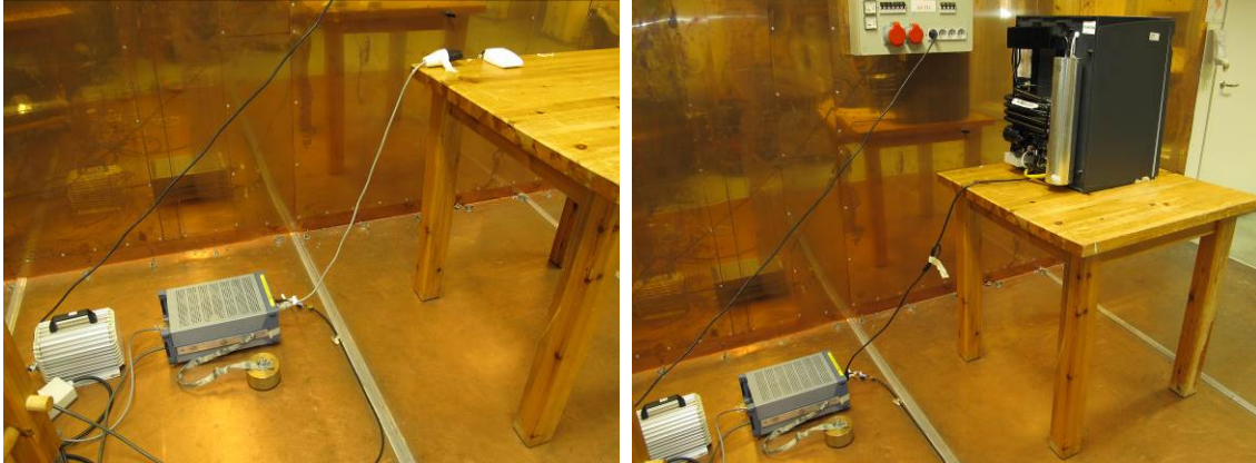
Conducted emissions measurements from AC mains
