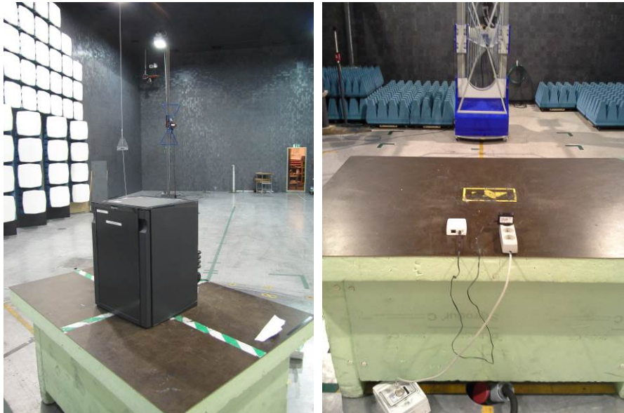
Radiated emissions measurements from 30 MHz to 1000 MHz
