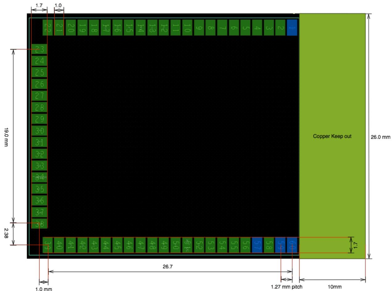
The module is a "solderable module and therefore the pad dimensions must be followed exactly.
