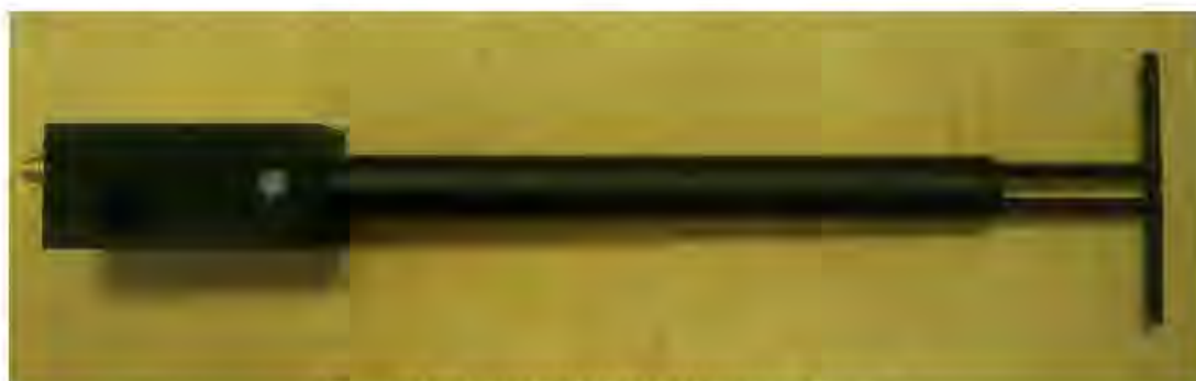
Figure 1 – MVG COMOSAR Validation Dipole
