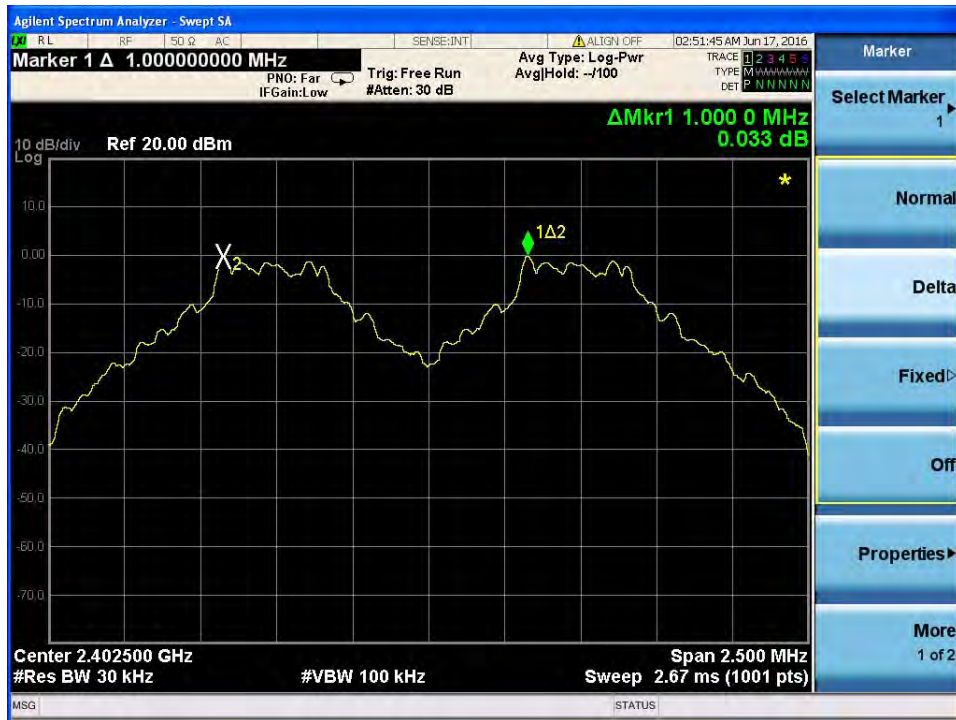
Channel Separation plot on channel 39-40
