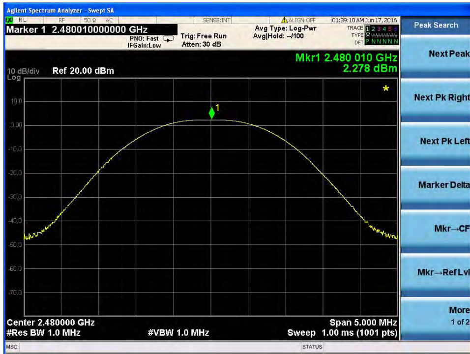
Peak output Power plot on channel 00
