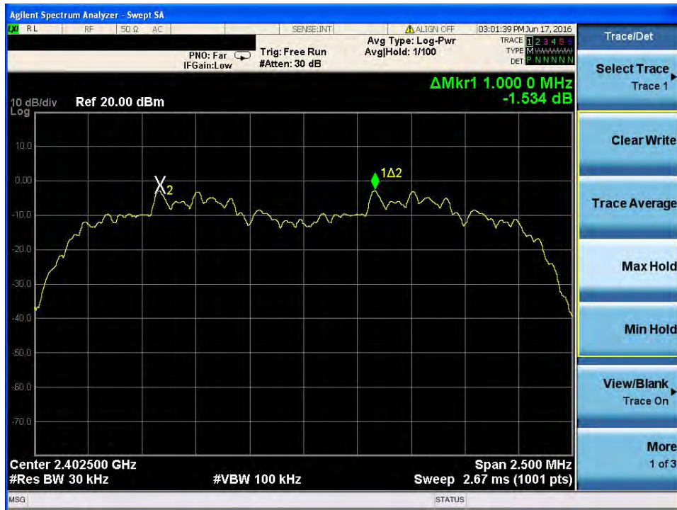
Channel Separation plot on channel 39-40
