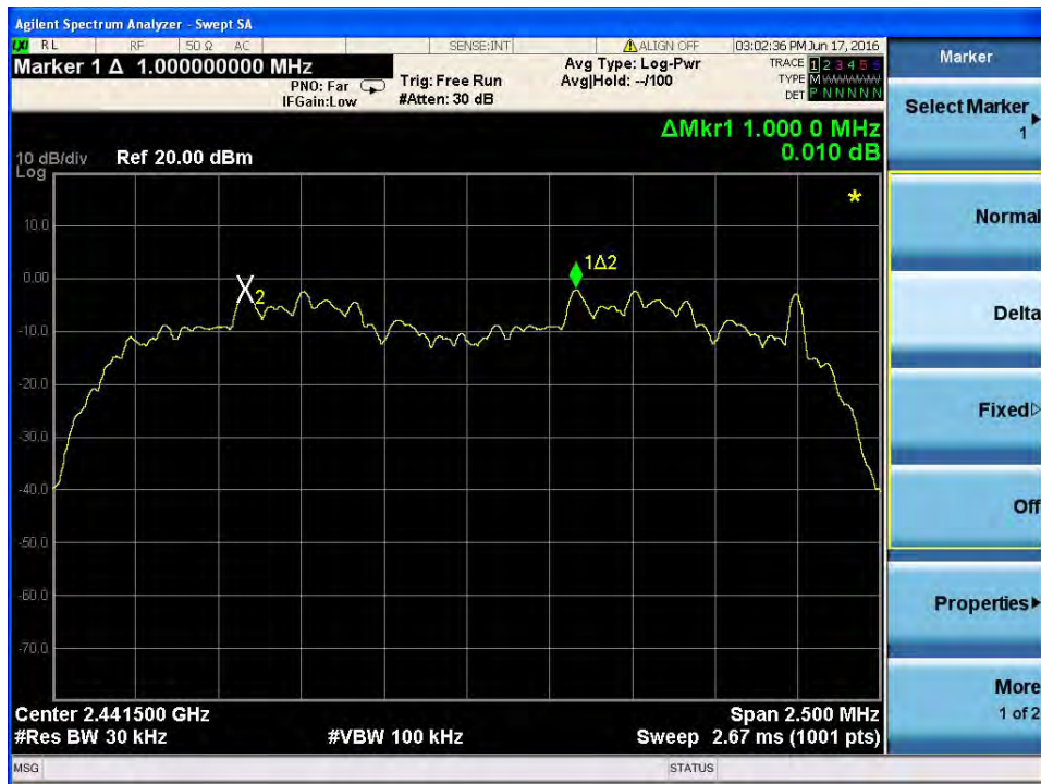
Channel Separation plot on channel 39-40
