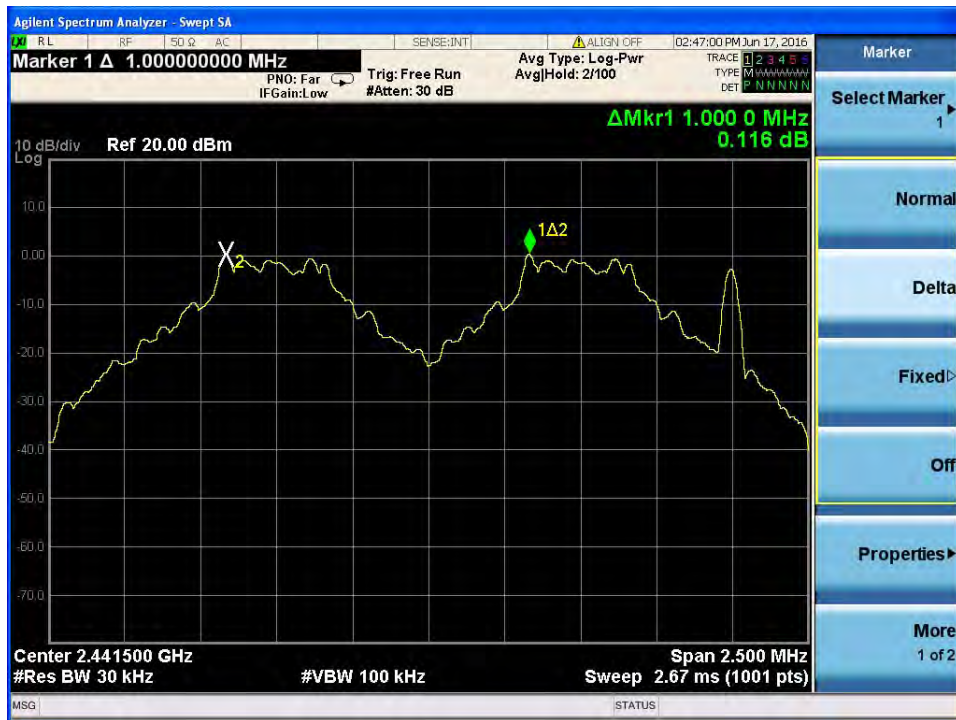
Channel Separation plot on channel 39-40
