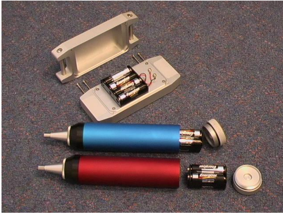
Figure 5. Probes and display unit opened for battery replacement
