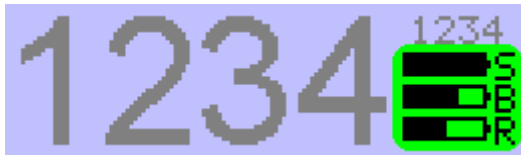
Figure 4. Battery life indicator portion of the display
