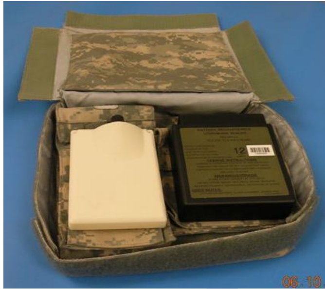
Figure 8. RDMS IPU Vehicle Pouch Showing the RDMS IPU and PATCO Battery
