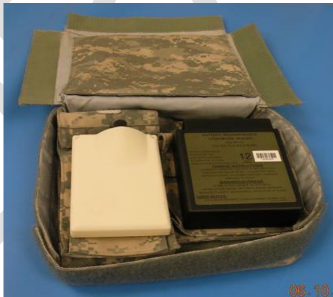
Figure 3. RDMS IPU Dismount Pouch showing the PATCO Battery
