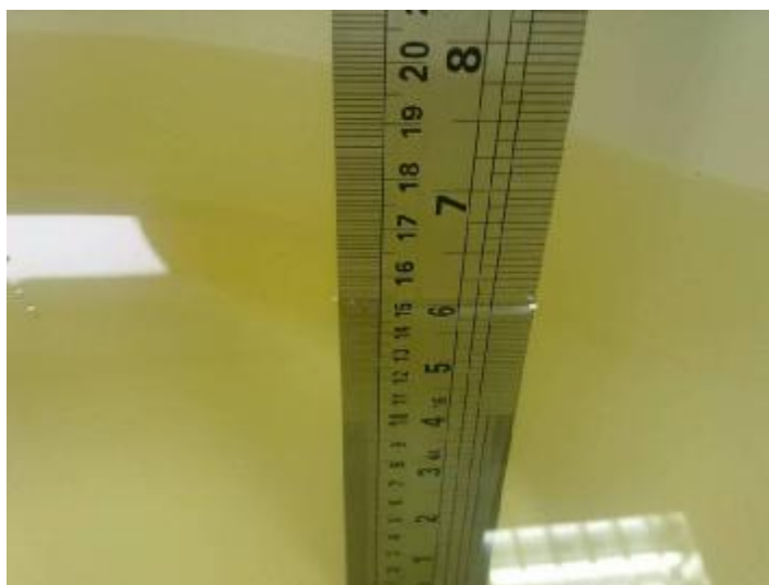
Photograph of the depth in the Body Phantom (2450MHz)
