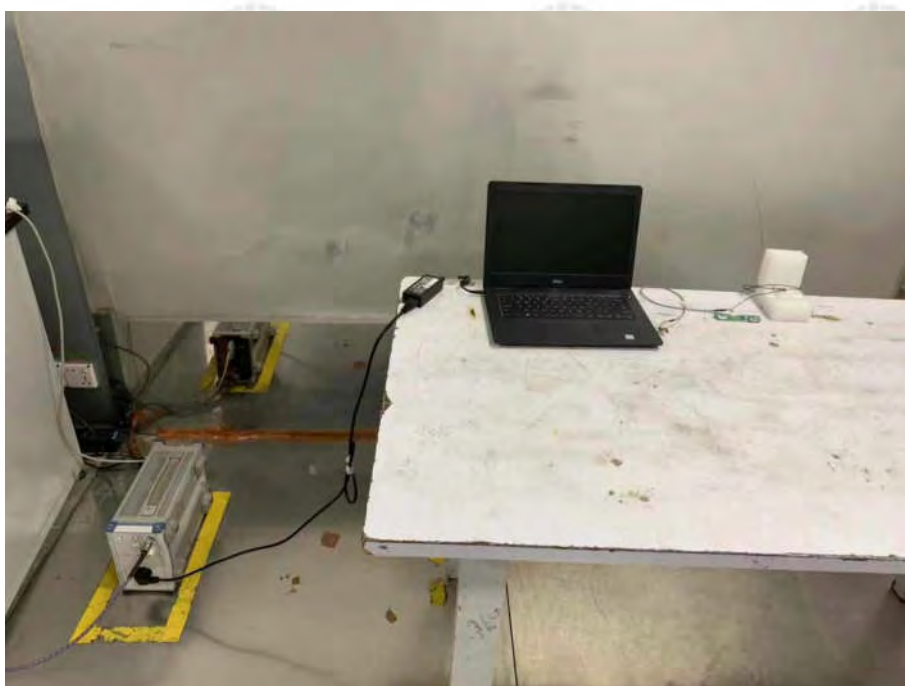
Conducted Emissions Test Setup
