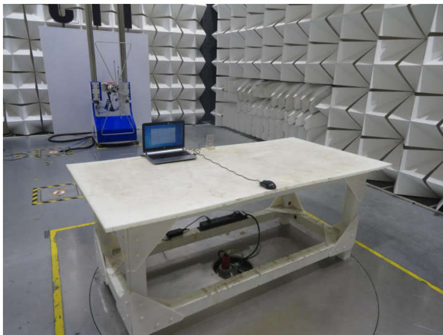
Radiated spurious emission Test Setup-2(30MHz-1GHz)
