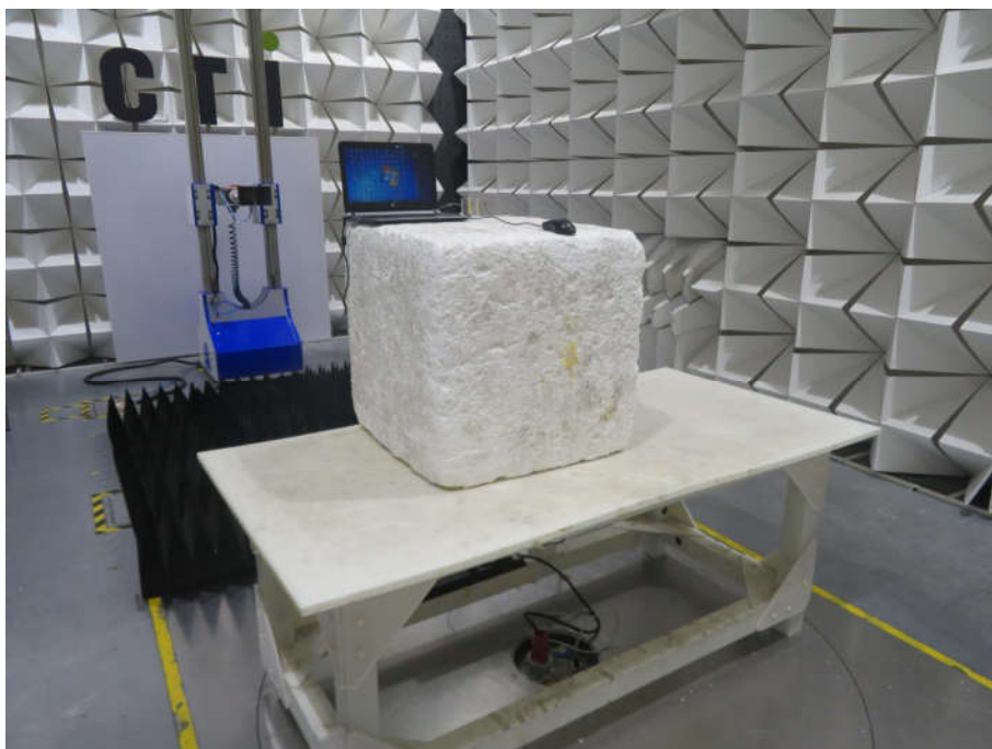
Radiated spurious emission Test Setup-3(Above 1GHz)
