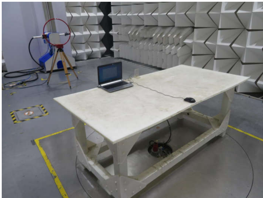
Radiated spurious emission Test Setup-1(Below 30MHz)
