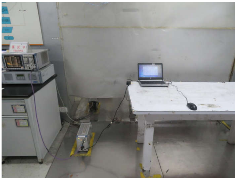
Conducted Emissions Test Setup
