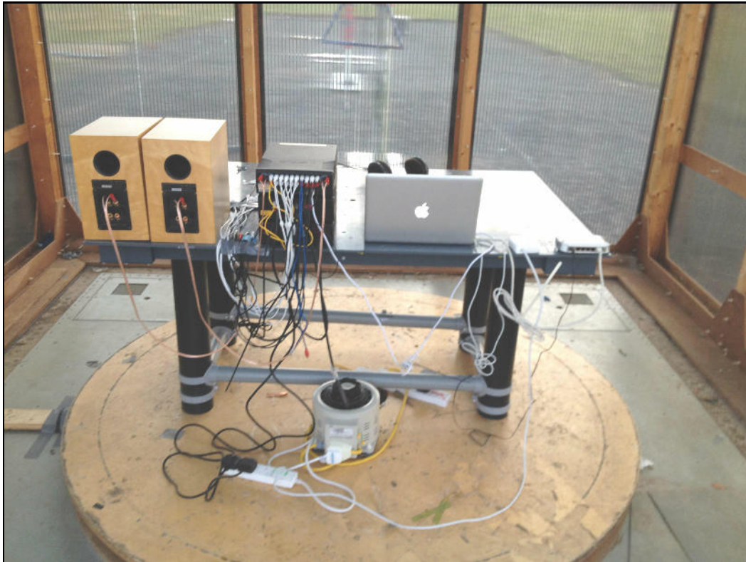
Photograph 11 Radiated Emissions - 6dac - USB Source
