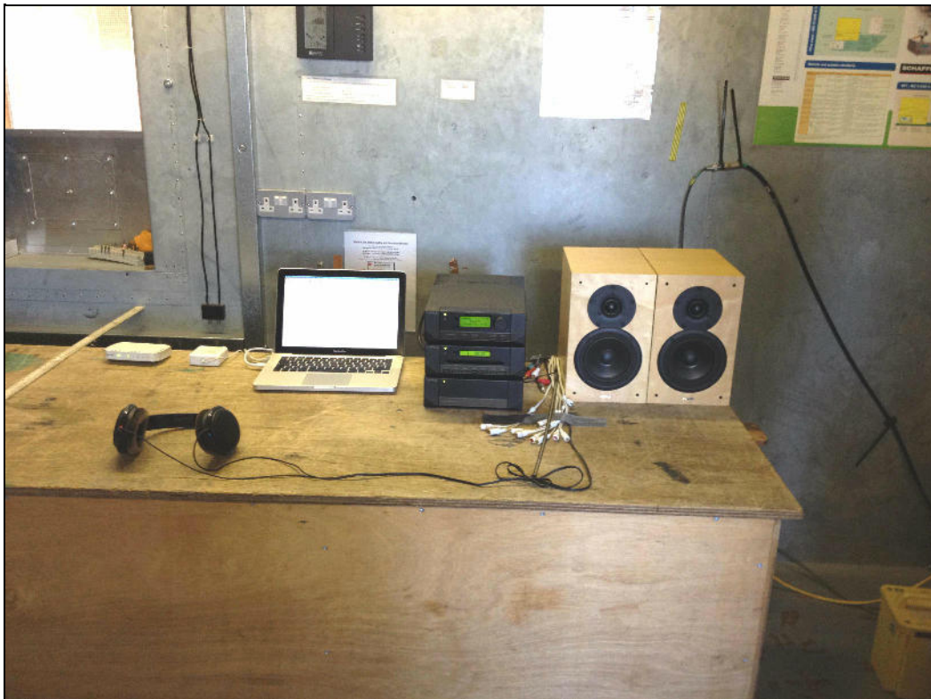
Photograph 4 Conducted Emissions - 8dac - USB Source
