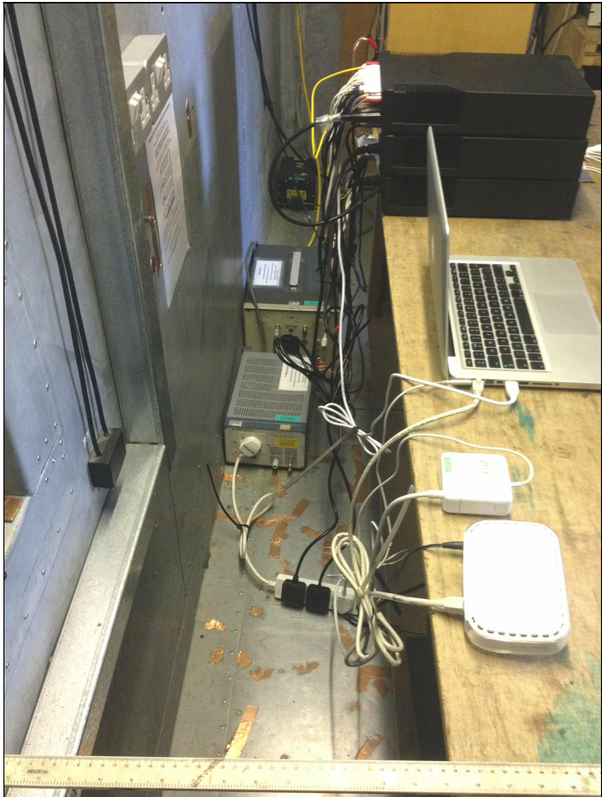
Photograph 8 Conducted Emissions - 6dac - USB Source
