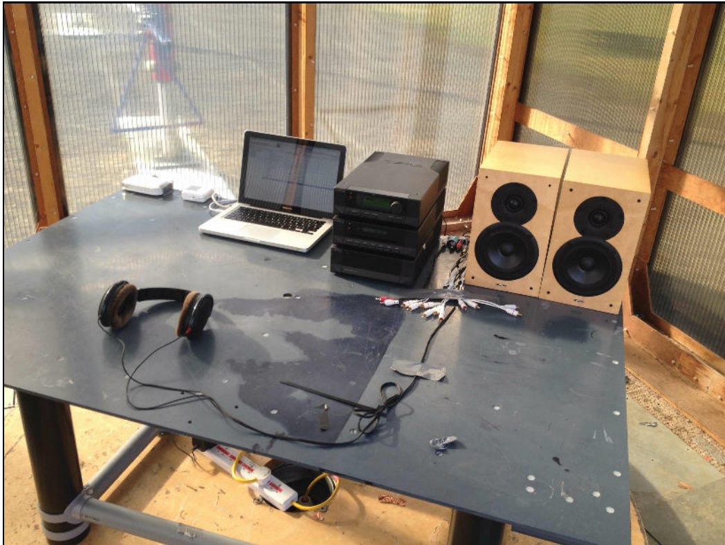
Photograph 9 Radiated Emissions - 8dac - USB Source
