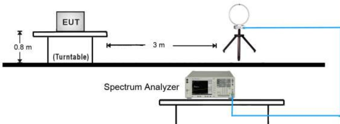
Below 1GHz Test Setup:
