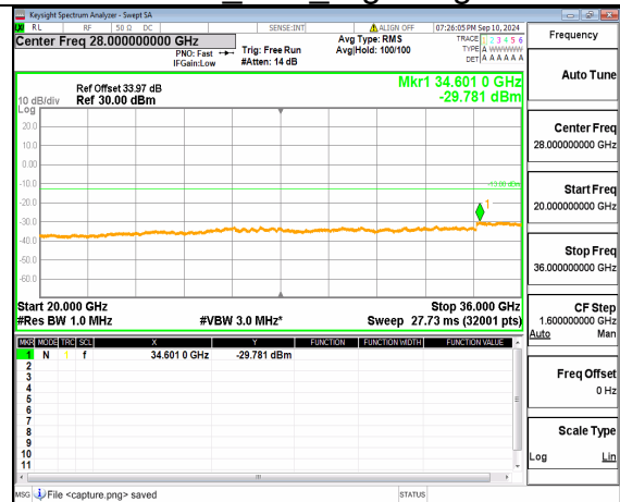
n77(3450-3550MHz) (20GHz-36GHz) 60M DFT-s-OFDM BPSK Inner_1RB_Left Low
