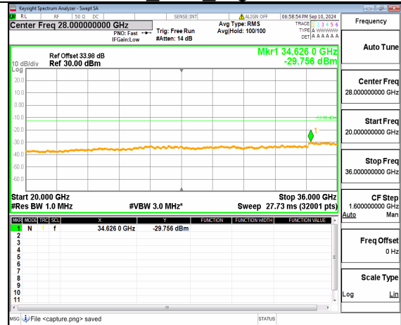
n77(3450-3550MHz) (20GHz-36GHz) 40M DFT-s-OFDM BPSK Inner_1RB_Left Mid
