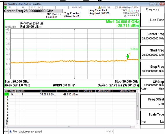
n77(3450-3550MHz) (20GHz-36GHz) 60M DFT-s-OFDM QPSK Inner_1RB_Left Low
