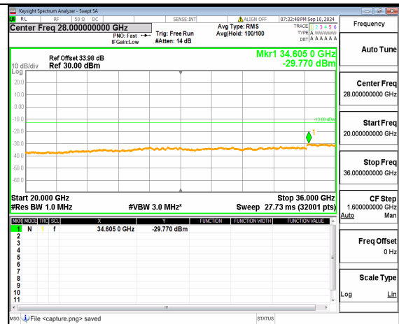
n77(3450-3550MHz) (20GHz-36GHz) 60M DFT-s-OFDM BPSK Inner_1RB_Right Mid
