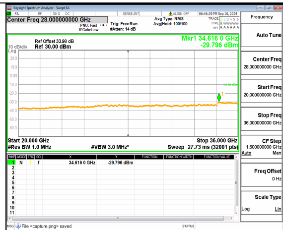
n77(3450-3550MHz) (20GHz-36GHz) 30M DFT-s-OFDM QPSK Inner_1RB_Right Mid
