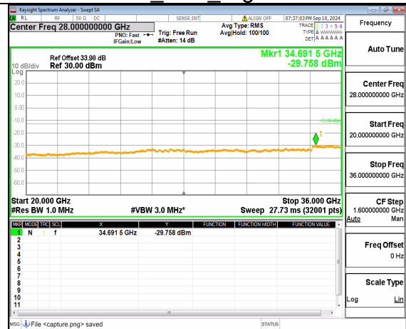
n77(3450-3550MHz) (20GHz-36GHz) 60M DFT-s-OFDM BPSK Inner_1RB_Left High
