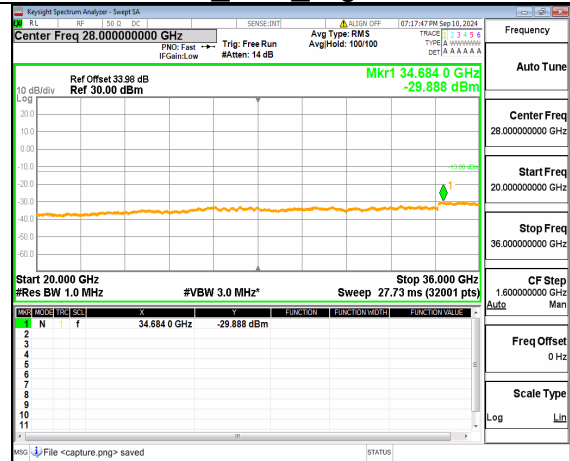
n77(3450-3550MHz) (20GHz-36GHz) 50M DFT-s-OFDM QPSK Inner_1RB_Left Mid
