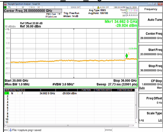
n77(3450-3550MHz) (20GHz-36GHz) 80M DFT-s-OFDM BPSK Inner_1RB_Left High
