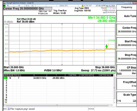
n77(3450-3550MHz) (20GHz-36GHz) 70M DFT-s-OFDM QPSK Inner_1RB_Left High
