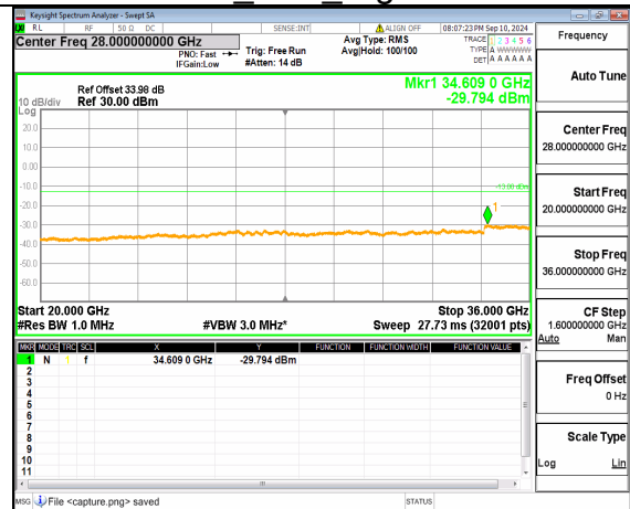
n77(3450-3550MHz) (20GHz-36GHz) 80M DFT-s-OFDM QPSK Inner_1RB_Left Mid
