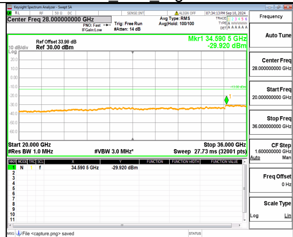
n77(3450-3550MHz) (20GHz-36GHz) 60M DFT-s-OFDM QPSK Inner_1RB_Left Mid
