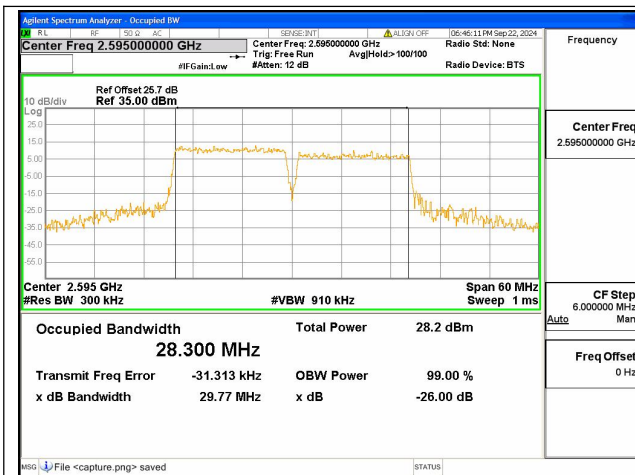
38C / 15+15MHz / 64QAM/ Mid CH
