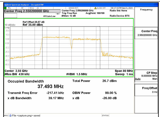
7C / 20+20MHz / 256QAM/ High CH
