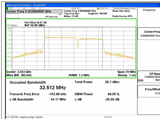
7C / 20+15MHz / 64QAM/ High CH
