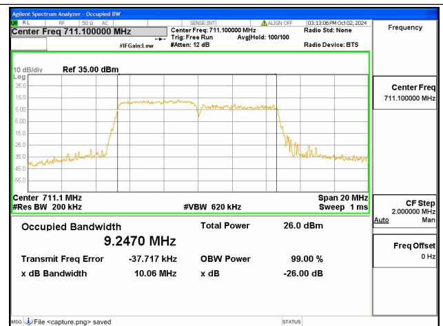
12B / 5+5MHz / 256QAM/ High CH
