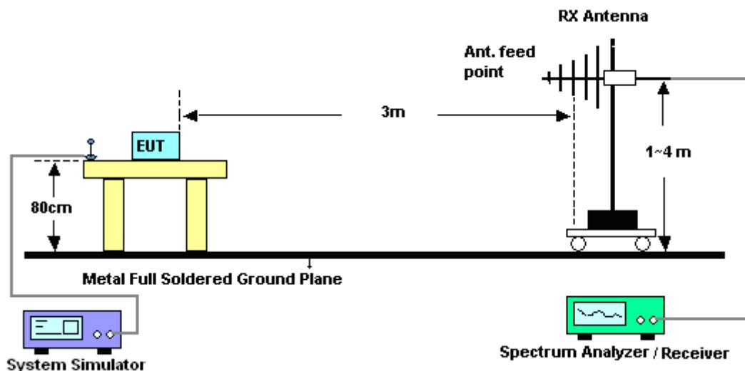
For radiated emissions from 1GHz to 18GHz
