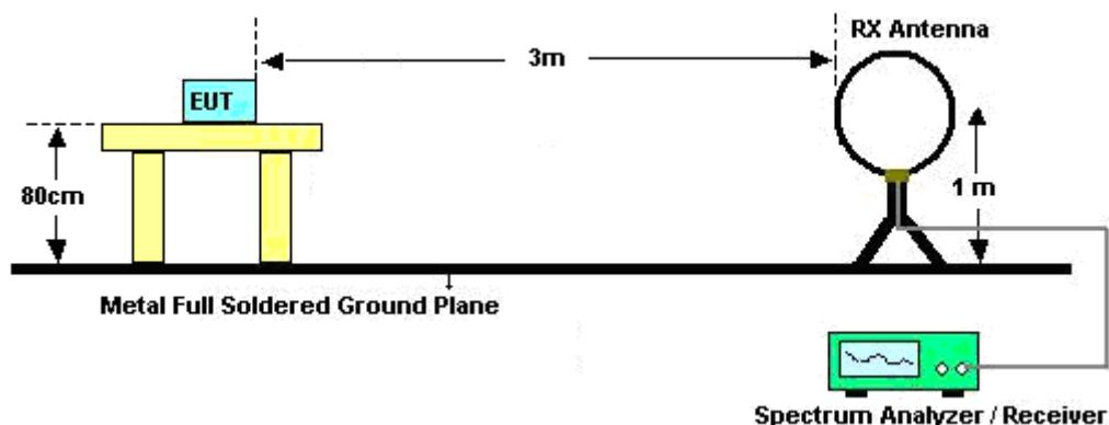
For radiated emissions from 30MHz to 1GHz
