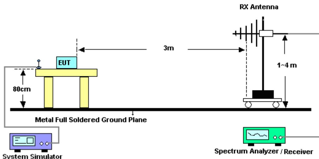
For radiated test above 1GHz
