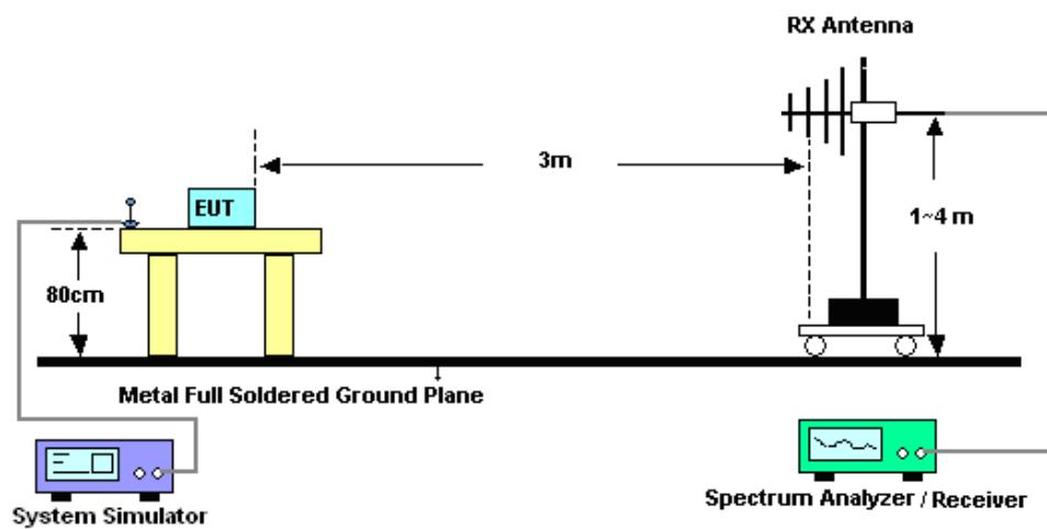
For radiated test above 1GHz
