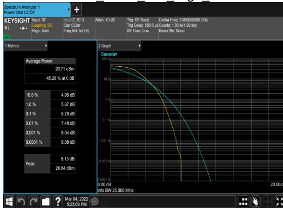
N77(20M)_DFT-s-OFDM_PI_2-BPSK Outer Full High CH
