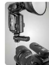
Turn off the camera. Insert the Hot Shoe Mounting Stand of the receiver into a camera hotshoe. Remove the hot shoe hatch of the camera. Insert one end of the Camera Remote Cable into "Camera Connection Port" of the receiver and the other end into the camera hot shoe port. Turn on the camera. Hold the transmitter in hand.
