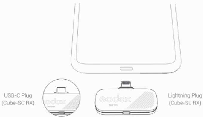
Connect the receivers Cube-SL RX and Cube-SC RX to power source with USB-A to USB-C cable and insert into smartphones, then they can charge the smartphone and be used at the same time.
